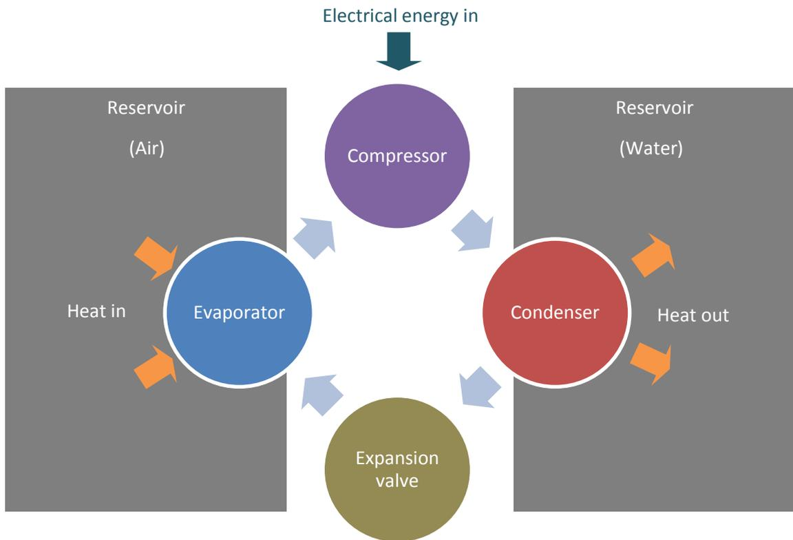
**Figure 1. Heat pump thermodynamic cycle**
