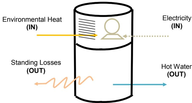
**Figure 2. Energy balances of a HPWH system**
