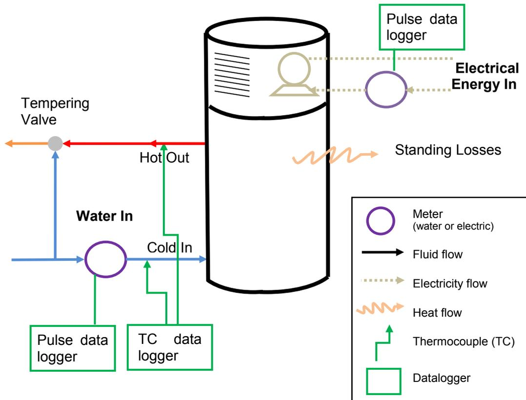
Figure 4. Monitoring arrangement for each HPWH
