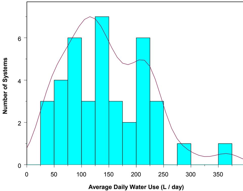
Figure 7. Histogram of average daily water use for 28 SWH systems, taken from Pollard and Zhao (2008) and the 11 HPWH systems examined in this project
