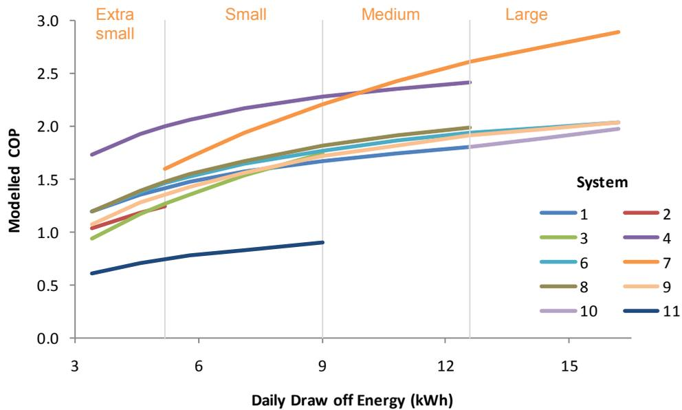
**Figure 10 Dependence of the modelled COP on the quantity of hot water draw off**
