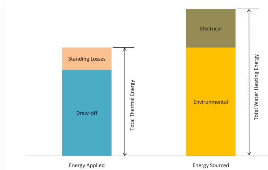
**Figure 3. An example of the energy balance of a HPWH system**
