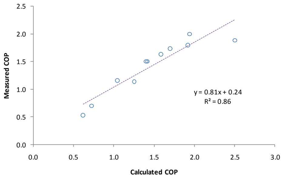
**Figure 8. Comparison of the calculated COP and measured COP for the HPWH systems**
