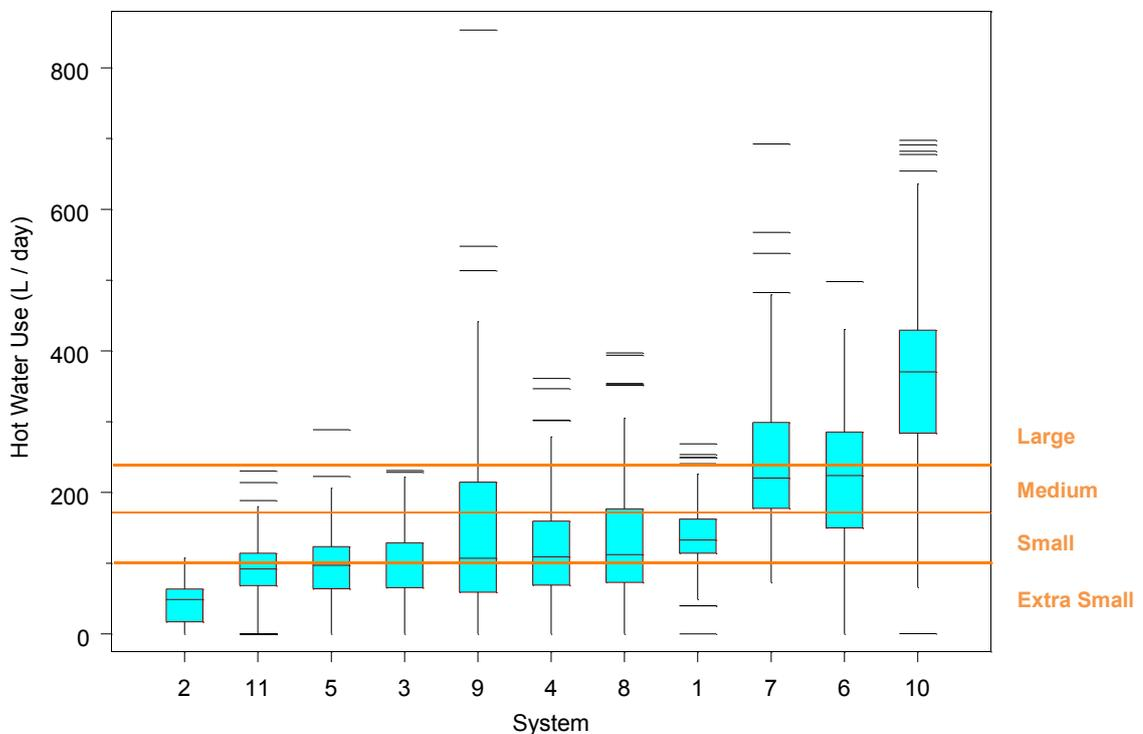
**Figure 6. Box plots of the daily water use for each of the HPWH systems**
