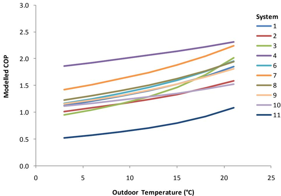
**Figure 9. Dependence of the modelled COP on the outdoor temperature for a small draw-off**
