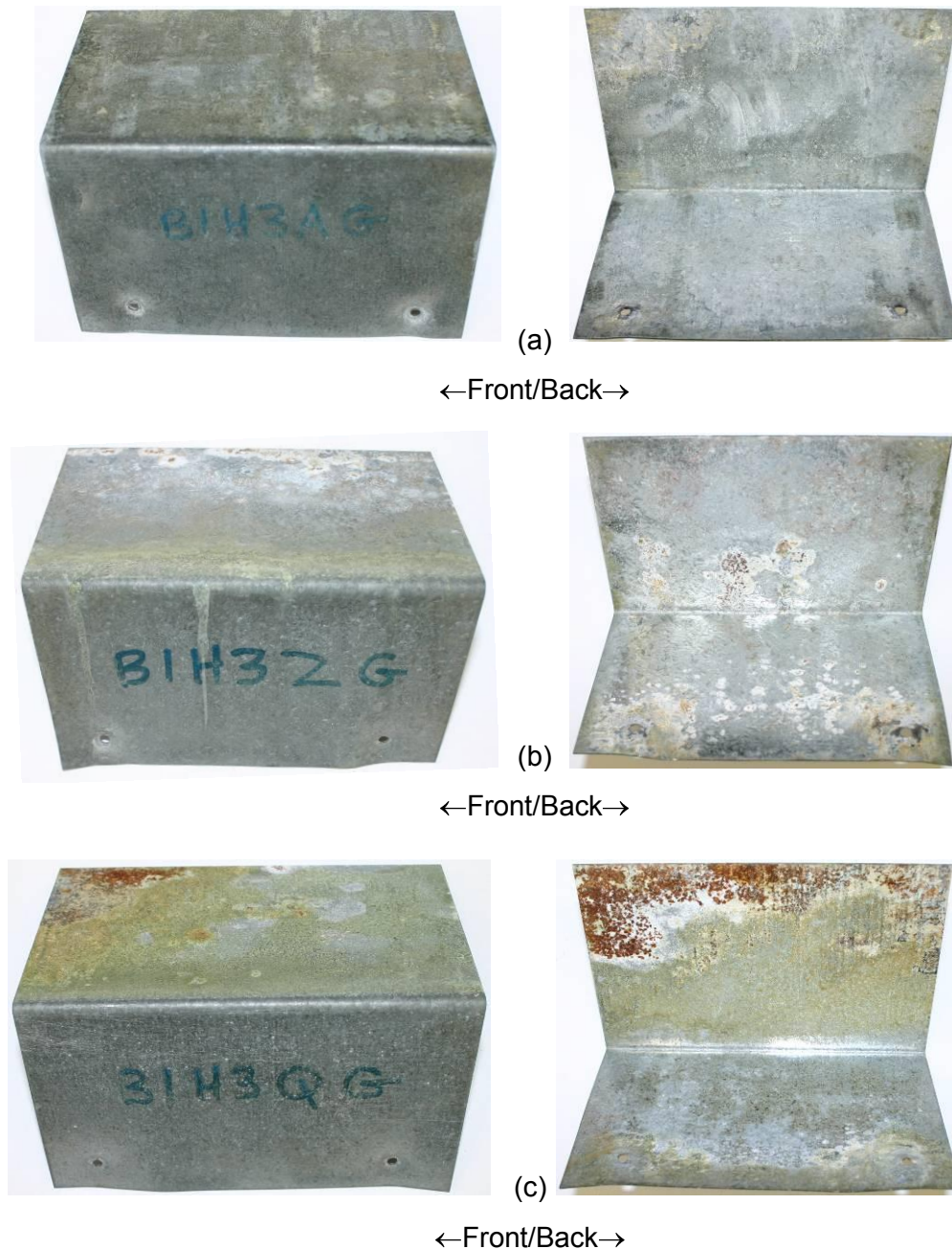
Figure 10: Surface morphology of hot dip galvanised steel flashing attached to timber exposed at Judgeford site for one year – (a) H3 CCA, (b) H3 CuAz and (c) H3 ACQ
