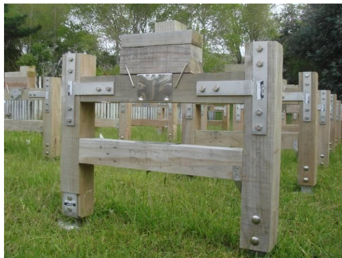
Figure 1: Photo of the gate-shaped timber structures, designed to incorporate a variety of metallic building fixings
