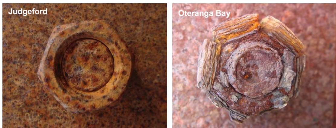
Figure 34: Mild steel nuts exposed at Judgeford and Oteranga Bay for three years
