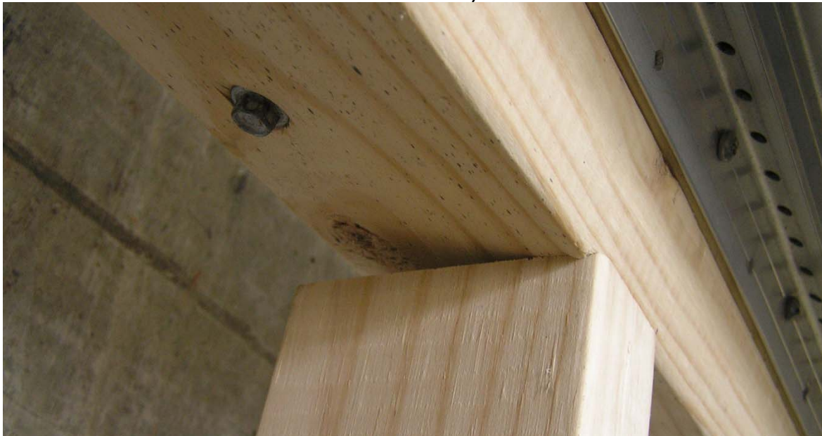
Figure 36. Twist of sill trimmer in Test 1 (photograph taken after the dummy sill section had been removed)
