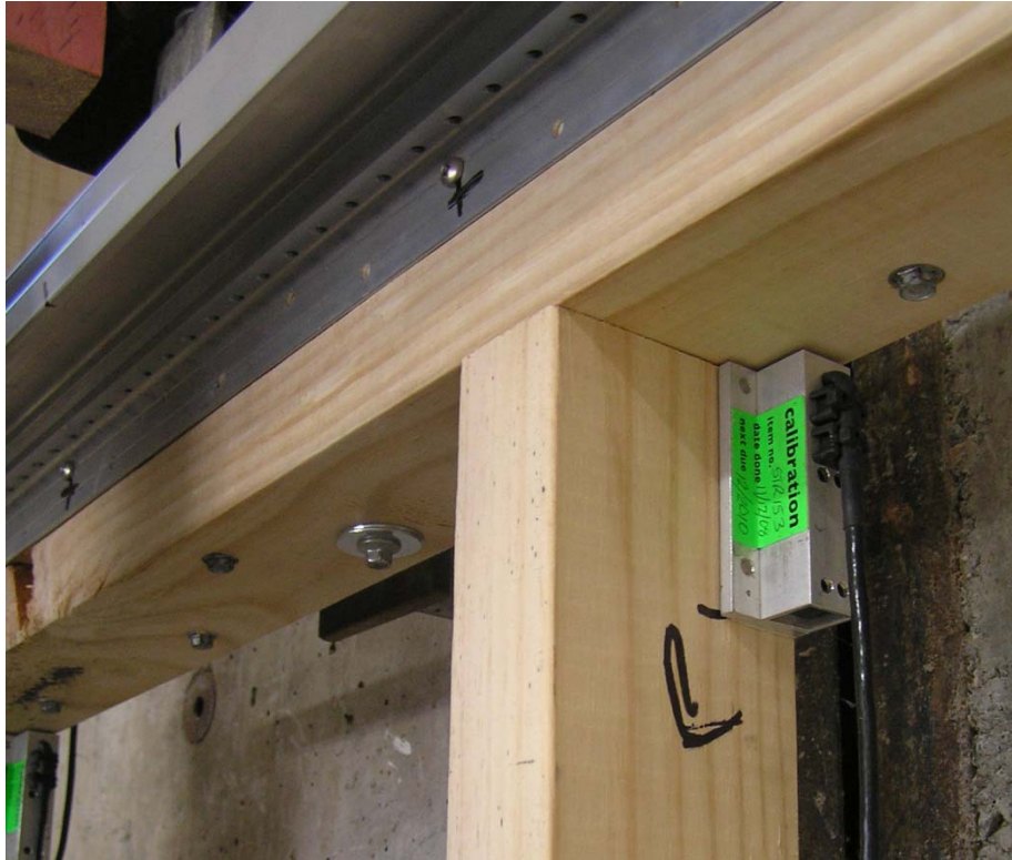
Figure 38. Test 2 deflection gauges and screw location
