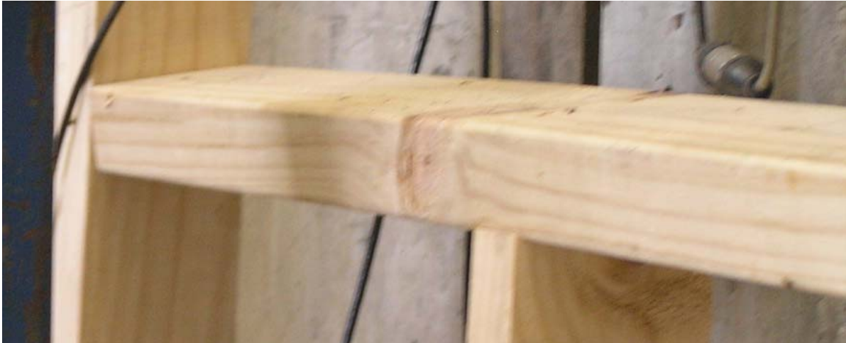
Figure 36. Twist of sill trimmer in Test 1 (photograph taken after the dummy sill section had been removed)
