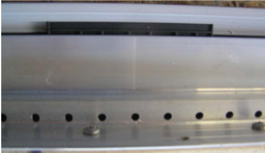
Figure 27. Pairs of screws at load location used in Test 1 (note the presence of the black window support block)
