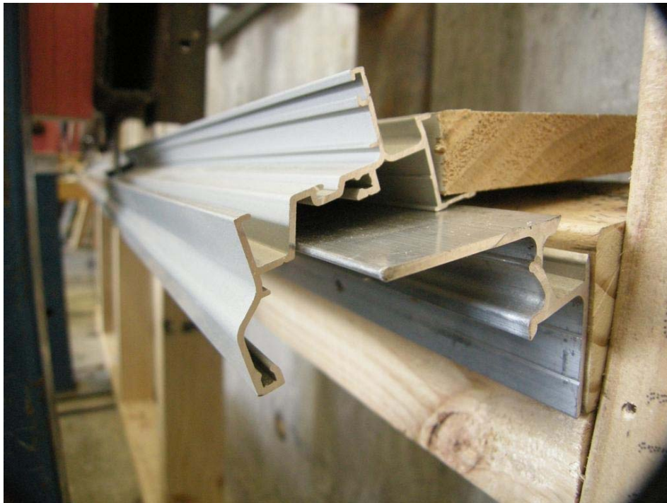
Figure 35. Distortion of the window frame and separation of frame and reveal at end of Test 1
