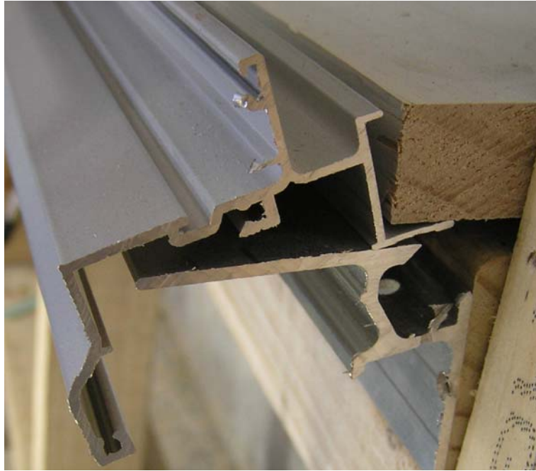
Figure 40. Test 2 frame off reveal and distortion observable at test completion
