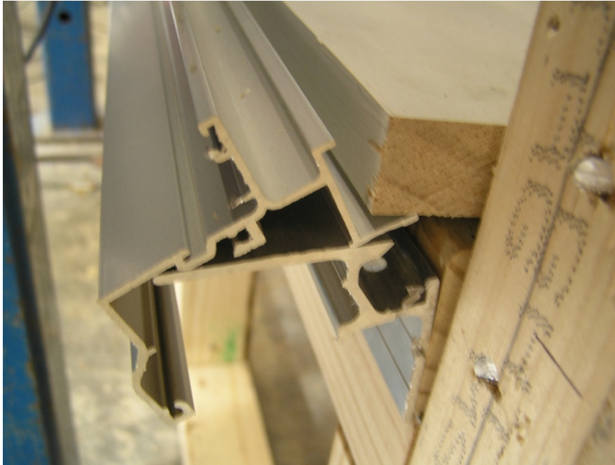
Figure 42. Cross-section at right-hand side of Test 3 at test completion
