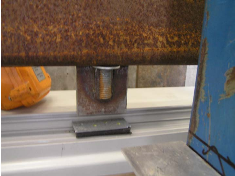
Figure 29. System to apply load onto steel plate covering the glazing setting block
