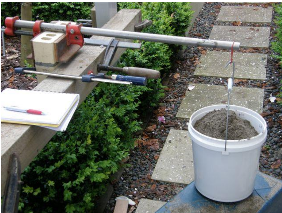
Figure 4. System for measuring bond strength from brick couplets in the greater Auckland region
