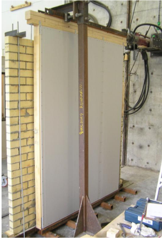
Figure 36. Test set-up for in-plane racking tests
