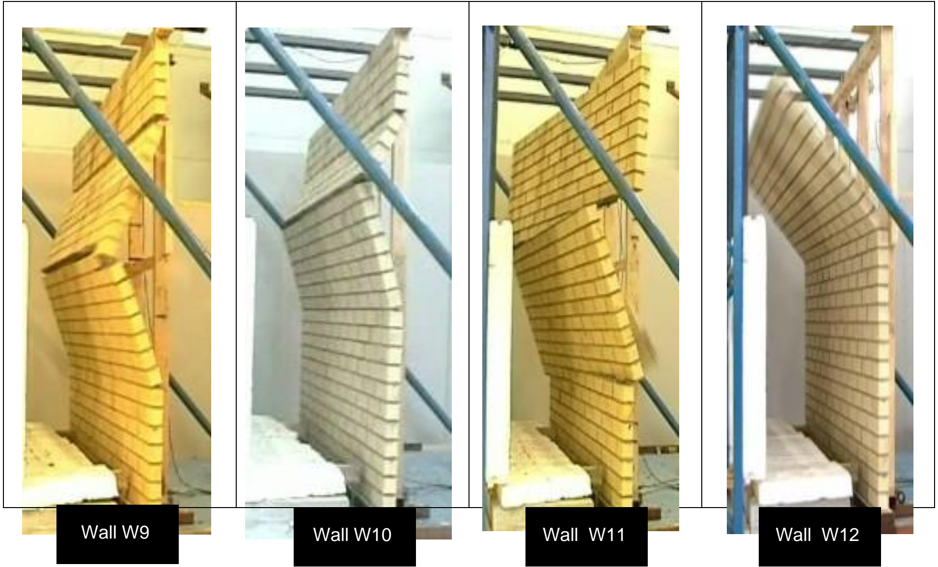
Figure 42. Photographs of veneer shedding mechanisms for the four test walls
