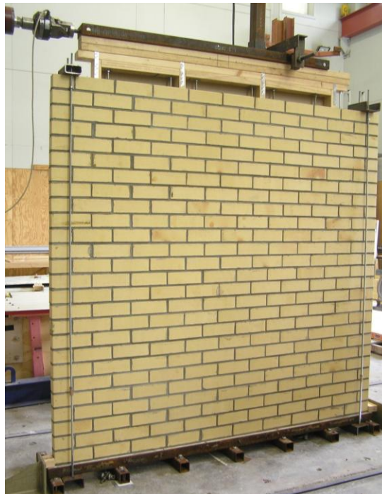
Figure 37. Test set-up for in-plane racking tests
