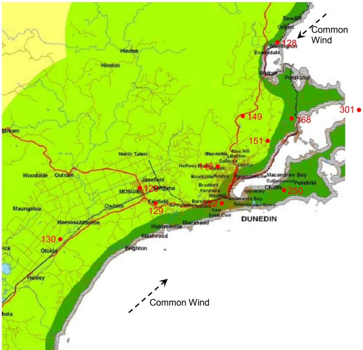
Figure 47. Corrosion zone boundary definition in NZS 3404 map for Otago region with mild steel corrosion rates derived from the present study (2011 – 2012)
