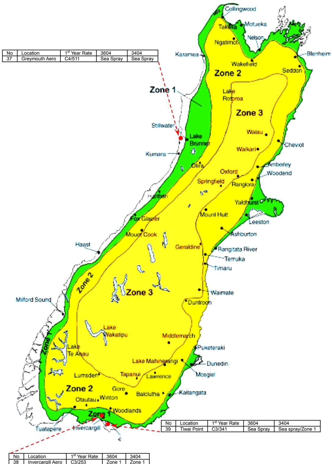
Figure 7. Atmospheric corrosion exposure sites in Greymouth and Invercargill regions
