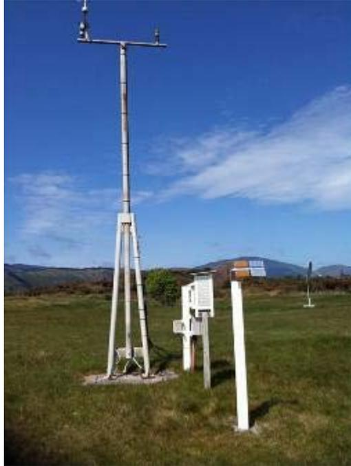
**Figure 8. Atmospheric corrosion exposure rack installed at MetService's weather station at Paraparaumu Airport**
