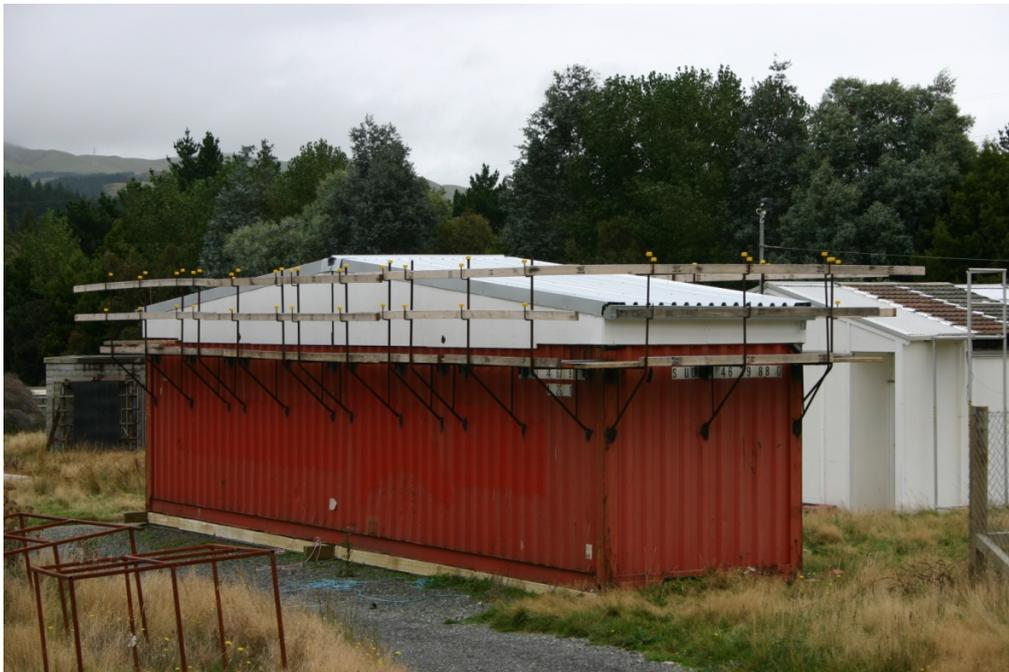
**Figure 5: Picture of the Roof Test Facility. We can see the container supporting the commercial roof specimen. Notice the plywood sheets closing off the side of the specimen. Also visible is the scaffolding used to work around the roof.**
