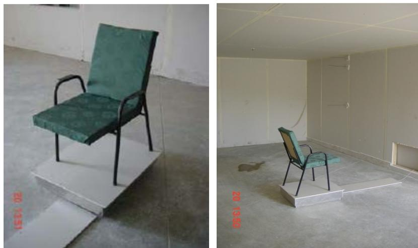
**Figure 48. Upholstered chair in centre fire position (extracted from Bittern, 2004)**
