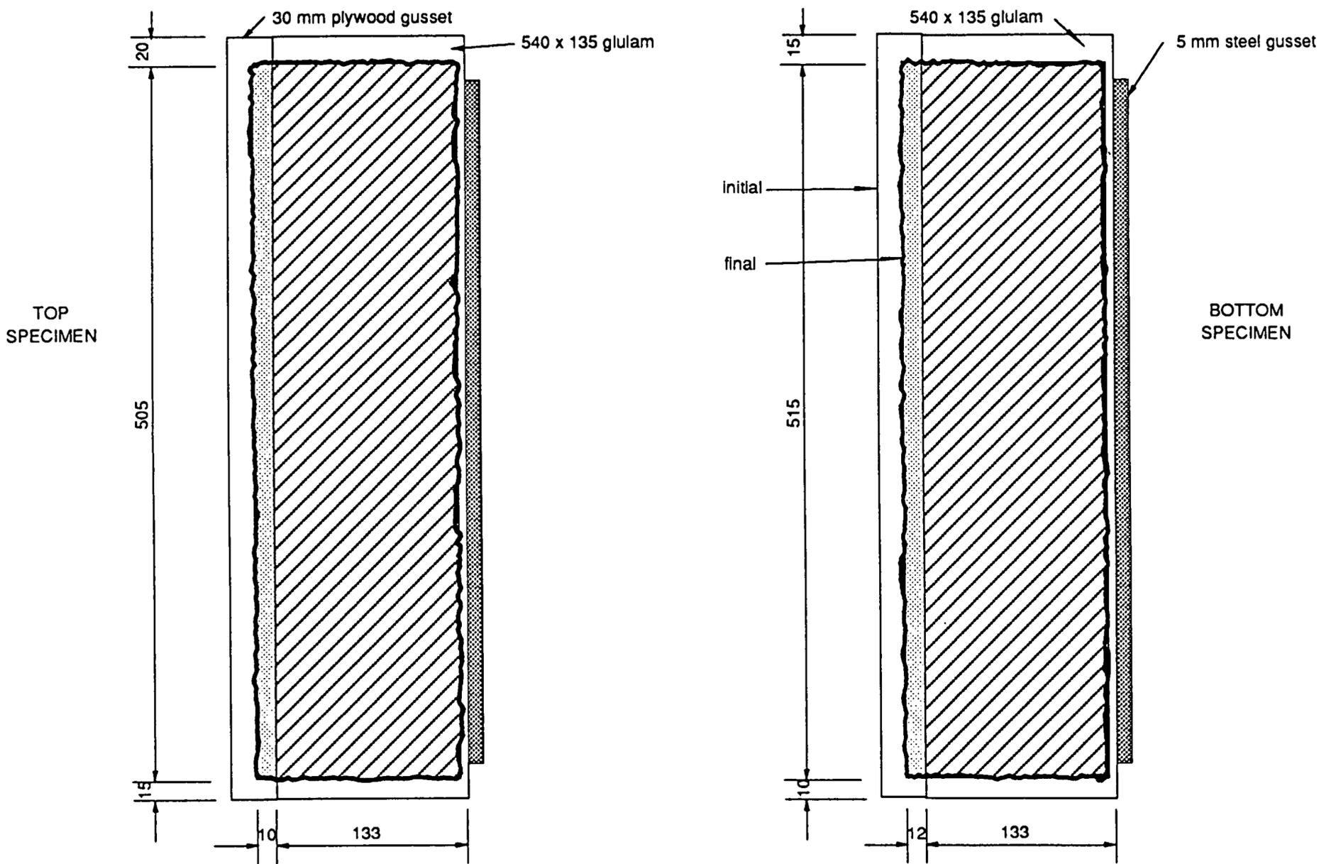
FIGURE 21a : Residual Sections of Test P1
