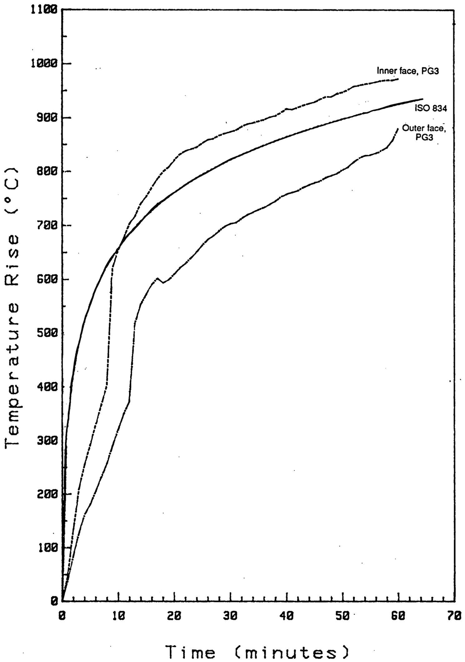
Figure 12: Furnace temperatures of joint PG3.
