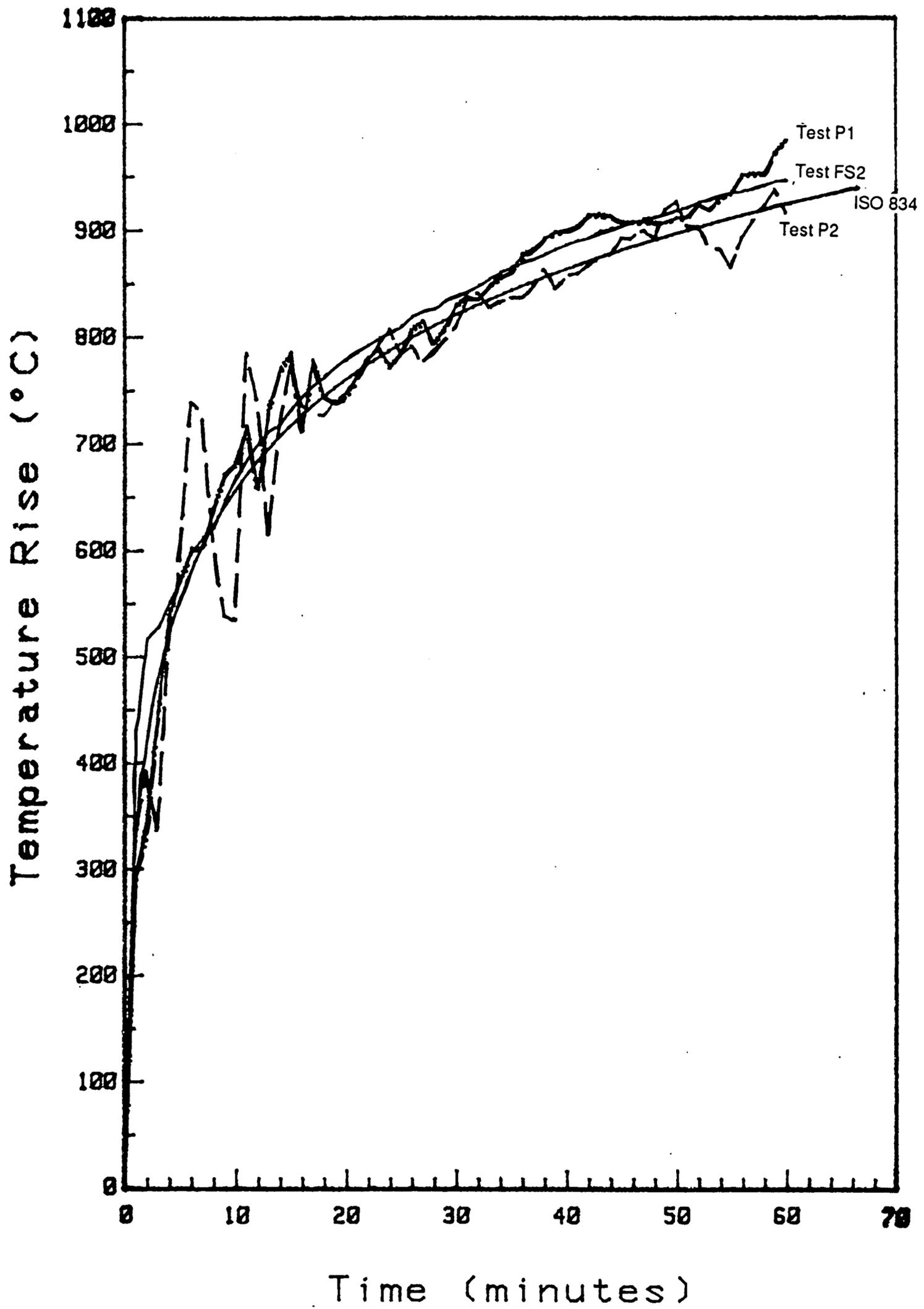
Figure 23: Comparison of average furnace and standard temperatures.
