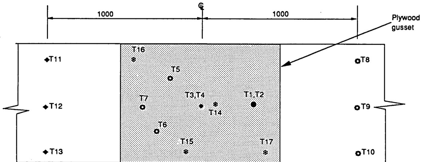
Figure 4a : Thermocouple Locations Test FS1
