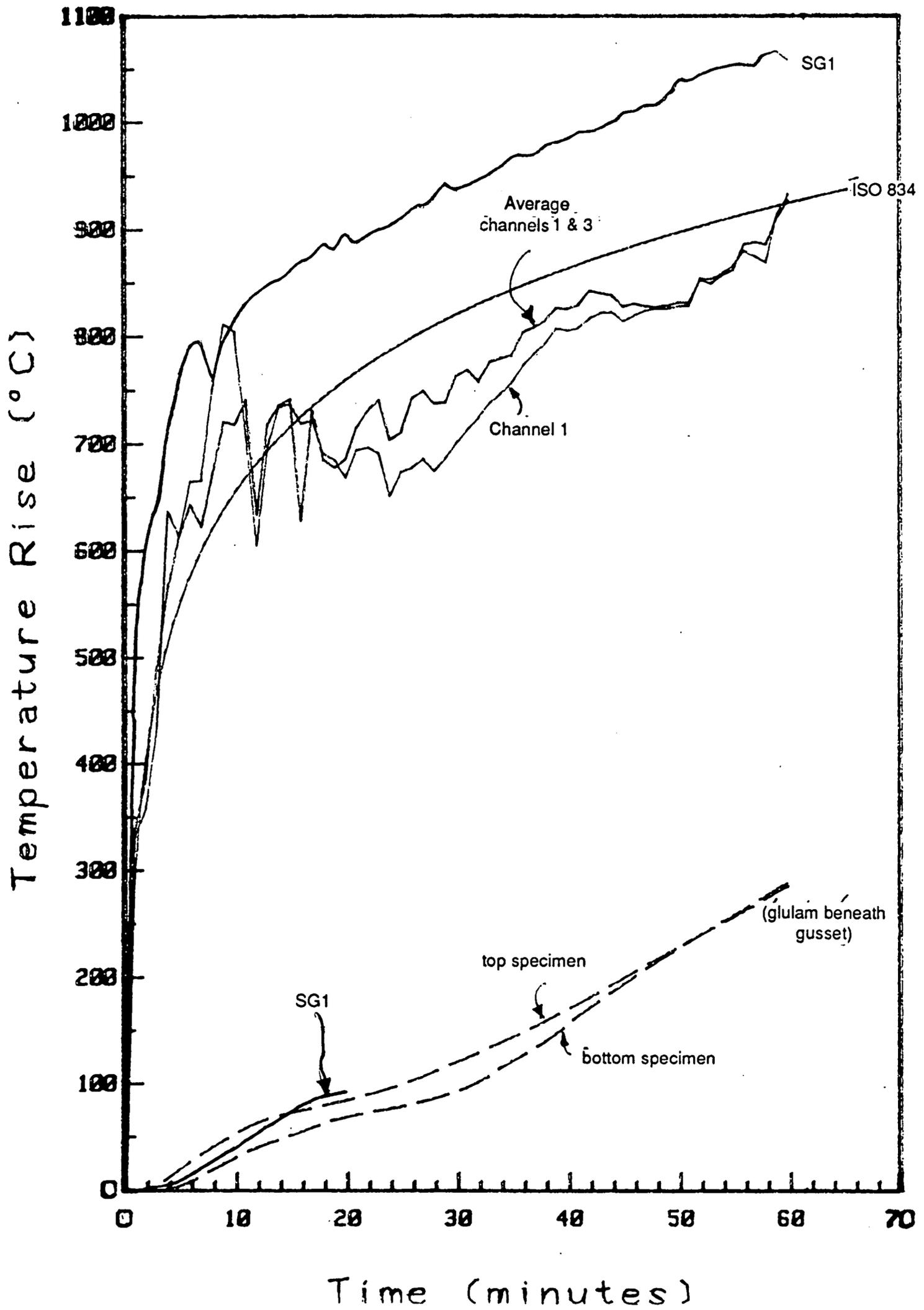
Figure 25a: Temperatures of steel specimens - test P1.
