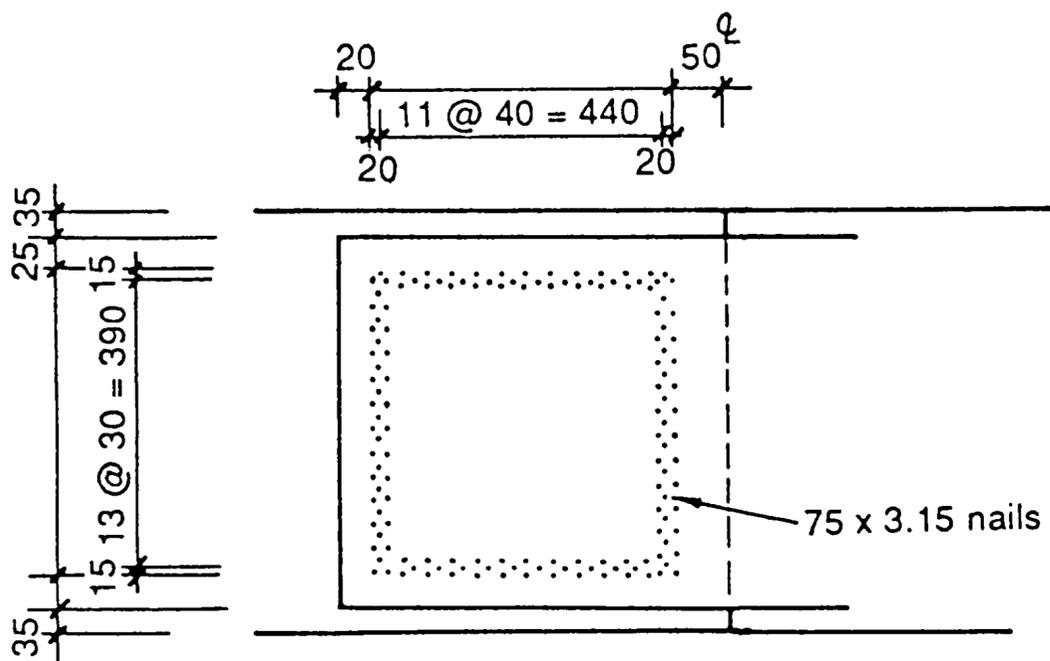
Figure 27b : 1100 x 470 x 5 steel gusset nailing pattern
