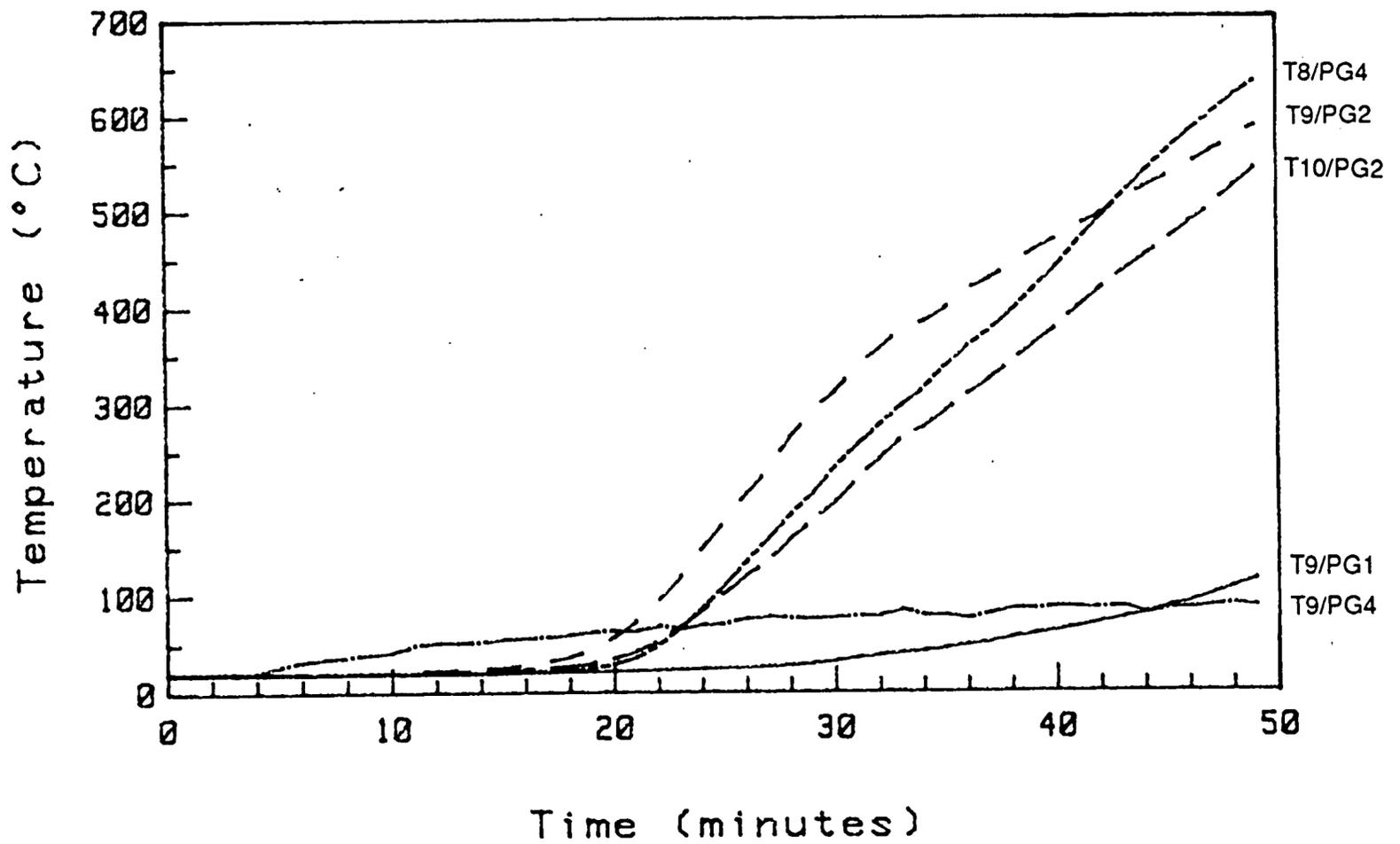
Figure 17a: Temperatures 67 mm into beam - test FS1.
