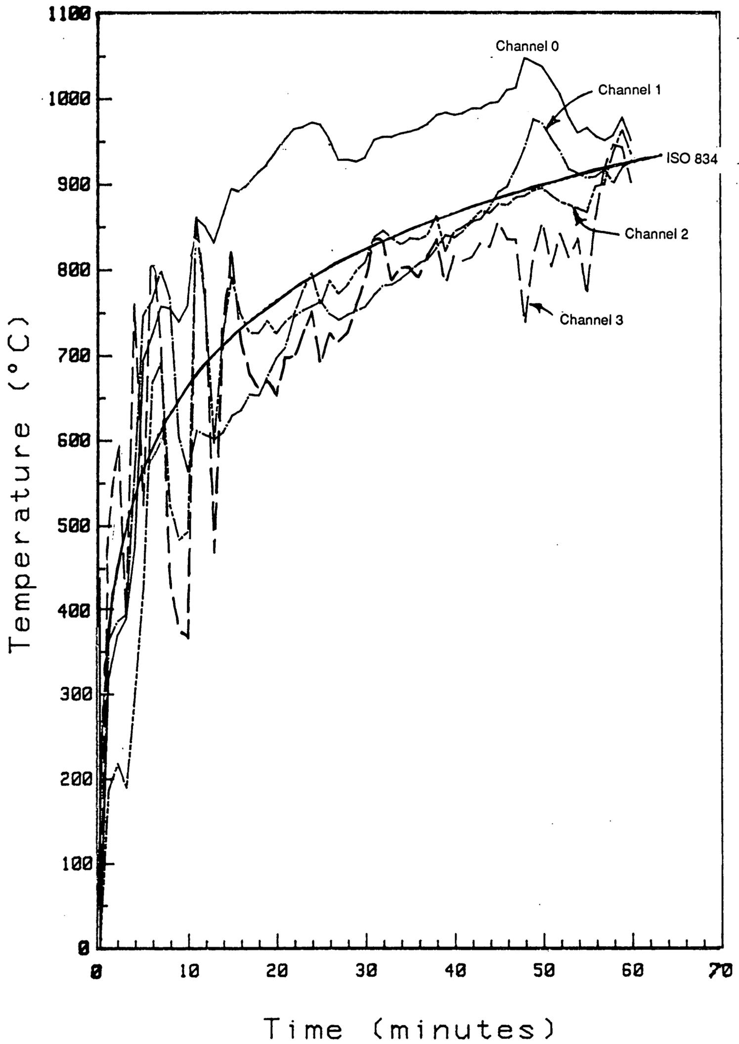
Figure 24b: Furnace temperatures - test P2.
