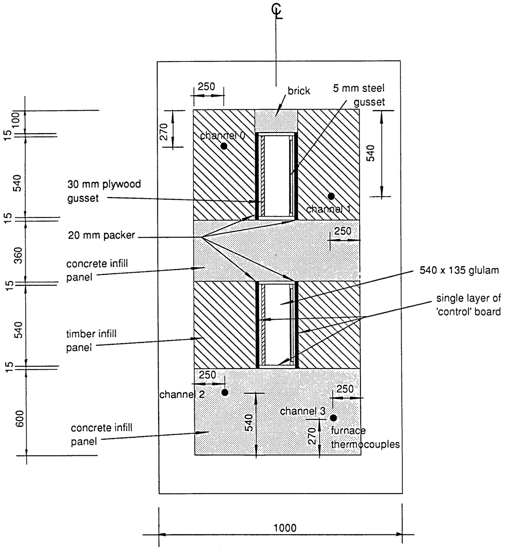
Figure 19 a : Elevation of Pilot Furnace Test P1. In Test P2, the Plywood Gussets Face the Other Wall.
