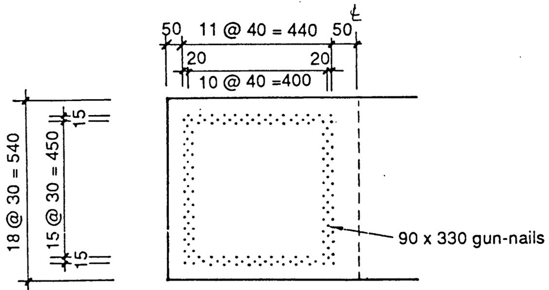
Figure 27a : 1100 x 540 x 30 plywood gusset nailing pattern
