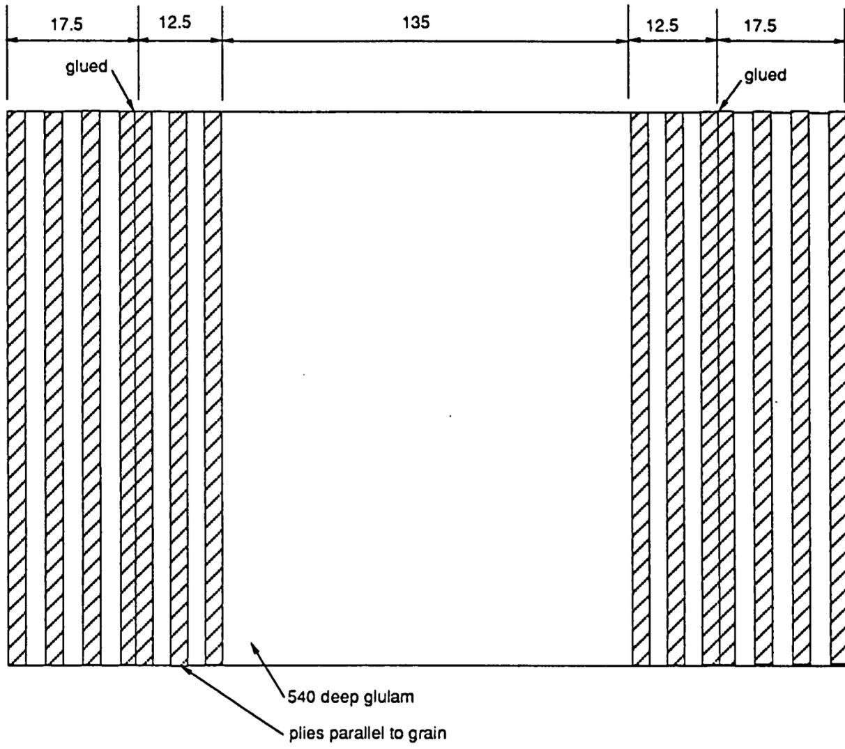
Figure 28 a : Plywood Gusset Before Test (N.T.S)
