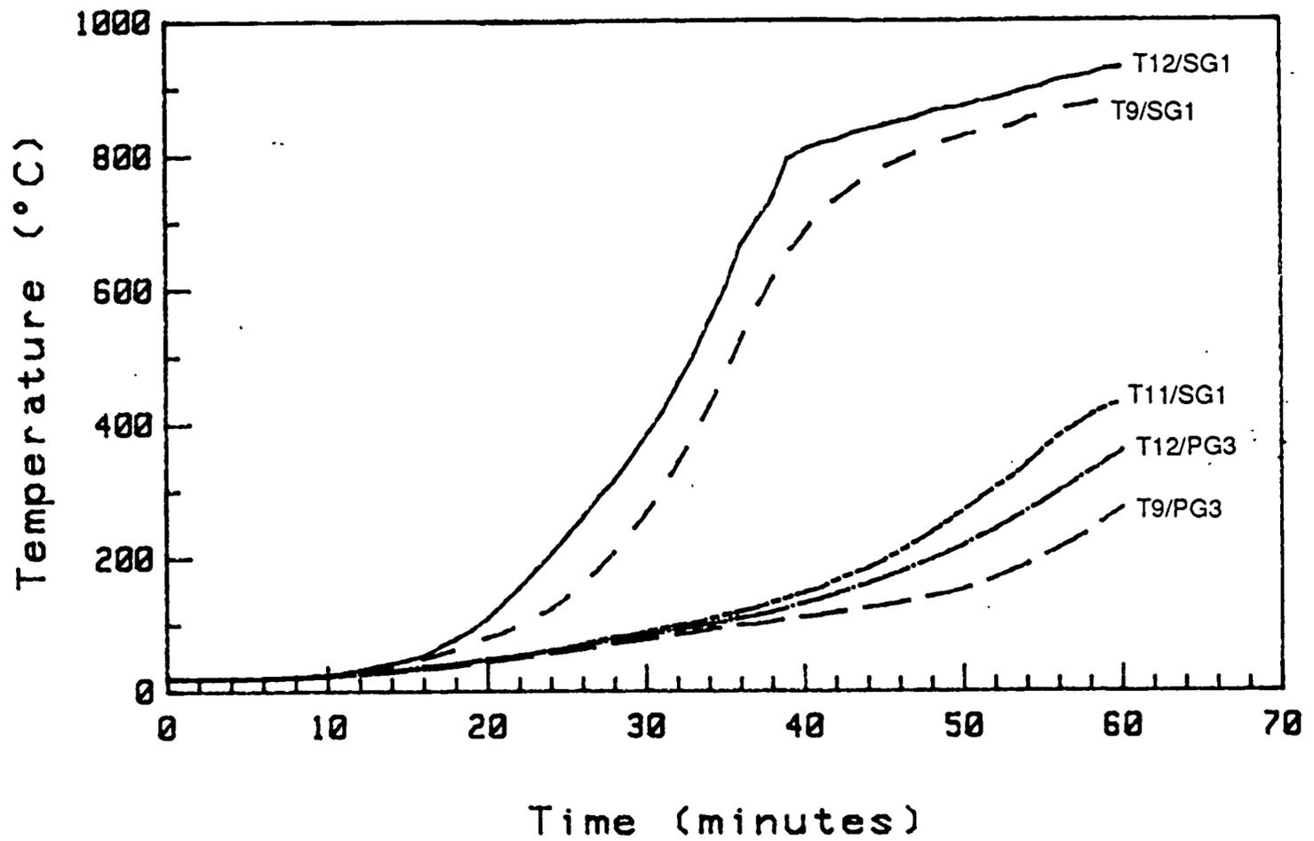
Figure 17b: Temperatures 45 mm into beam - test FS2.
