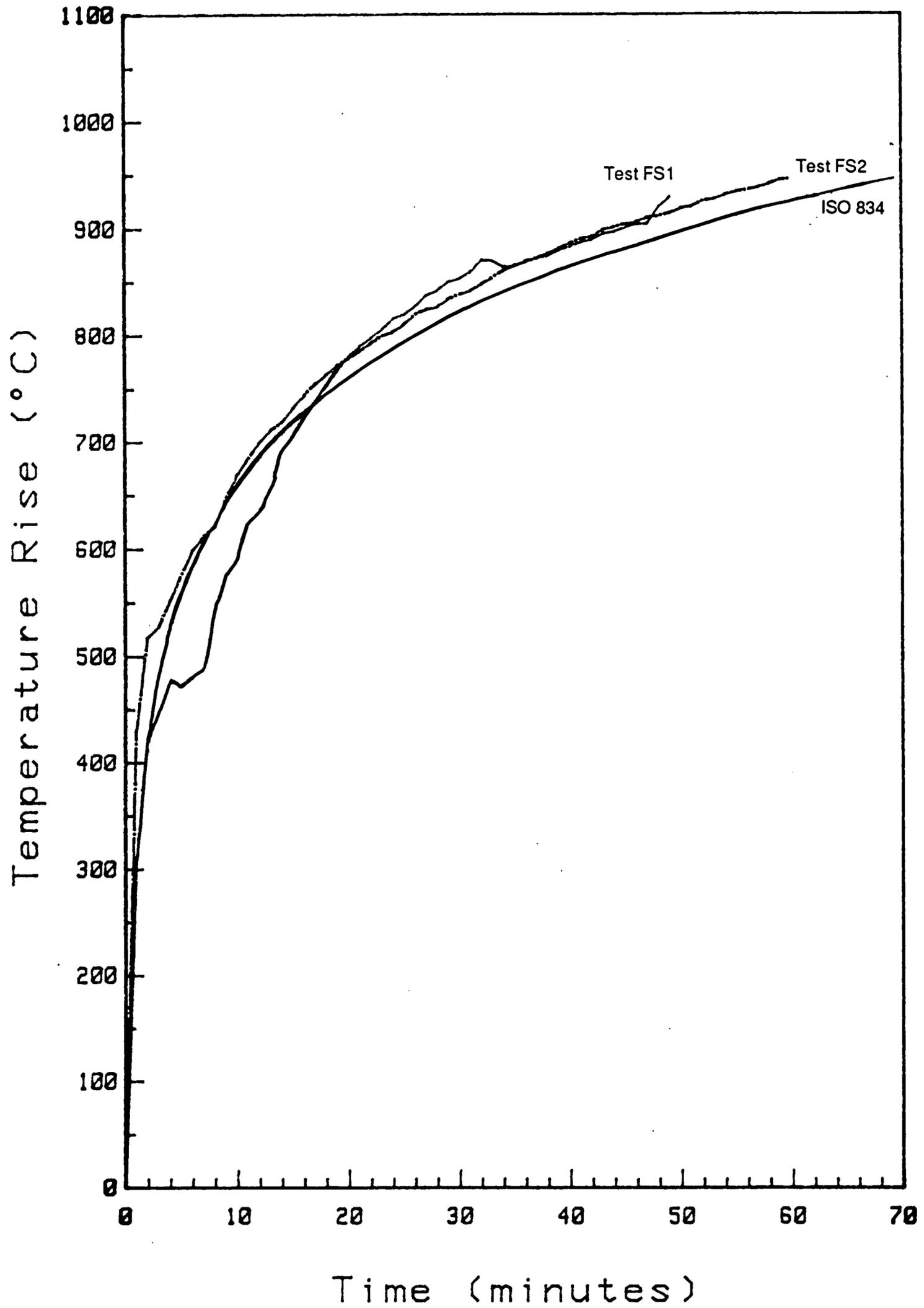
Figure 10: Comparison of average furnace and standard temperatures, tests FS1 & FS2.
