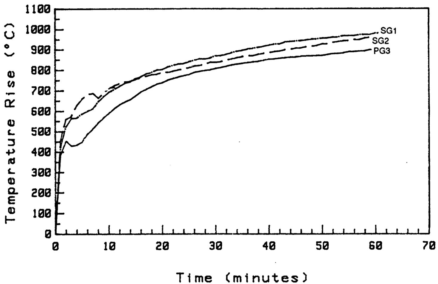
Figure 11b: Furnace temperatures 100 mm below beams, test FS2.
