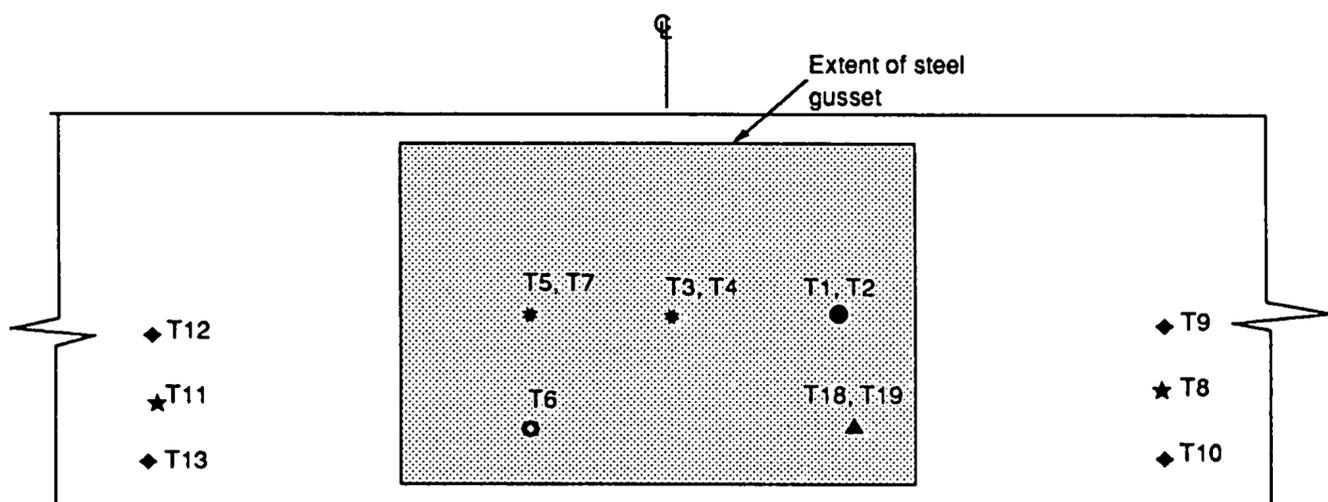
Figure 4b : Thermocouple Locations Test FS2
