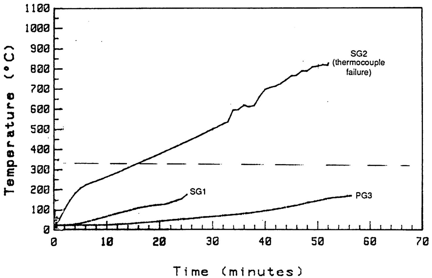
Figure 13b: Temperatures on beam surface beneath gussets, test FS2.
