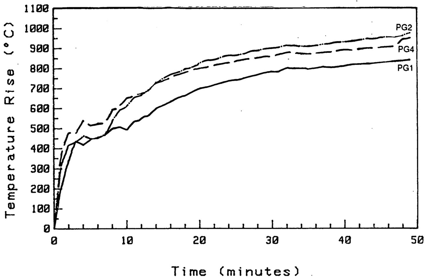
Figure 11a: Furnace temperatures 100 mm below beams, test FS1.
