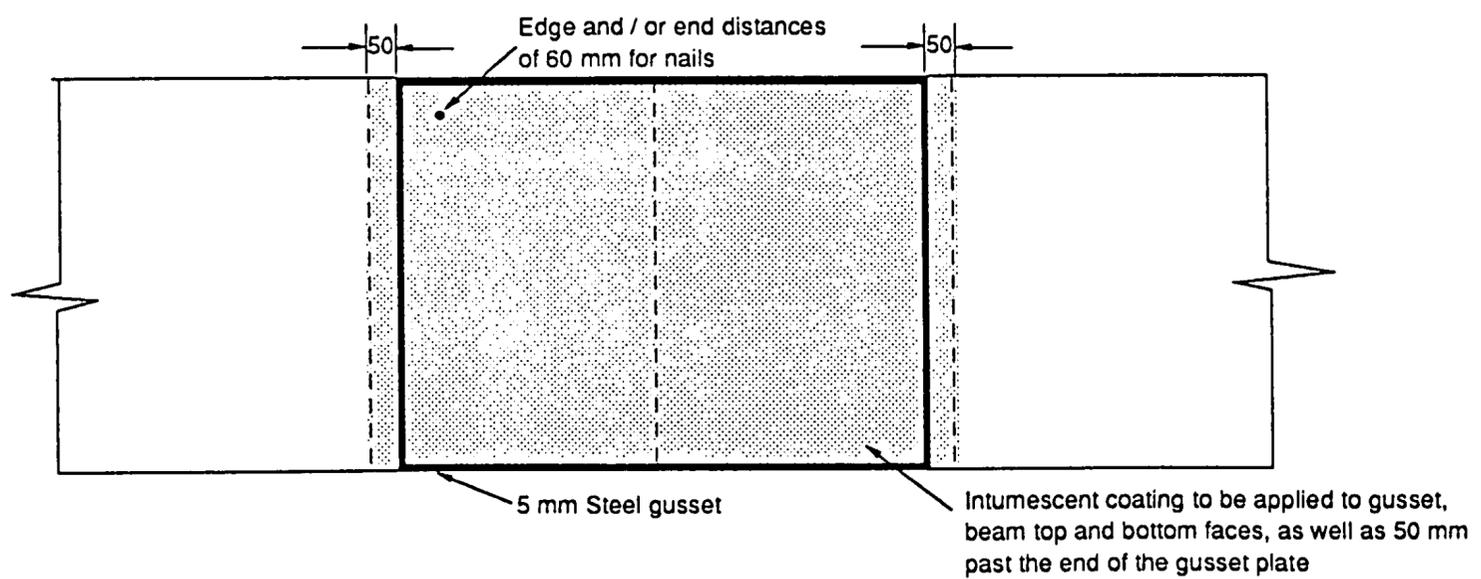
Figure 16b : Suggested detailing of gusset with Intumescent coating
