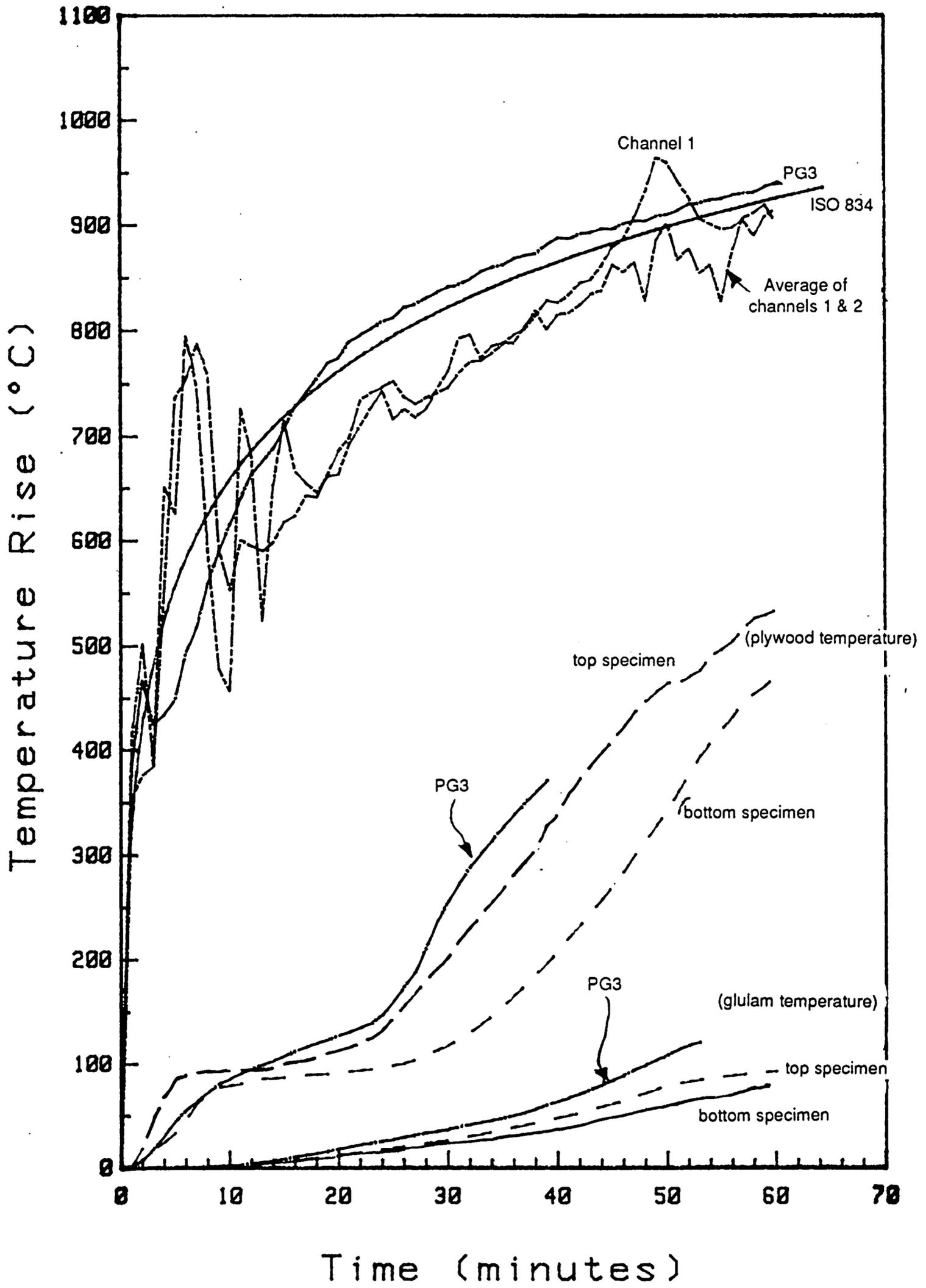
Figure 26b: Temperatures of plywood specimens - Test P2.
