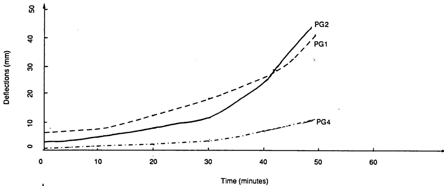
Figure 14a : Midspan Deflections Test FS1
