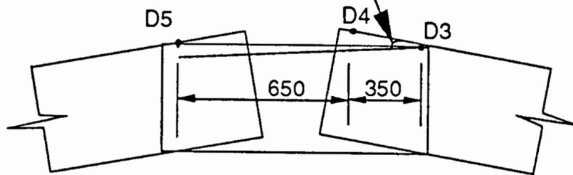
Figure 15a : Deformed Joint (exaggerated deformation) D3, D4, D5, are deflection measurement point
