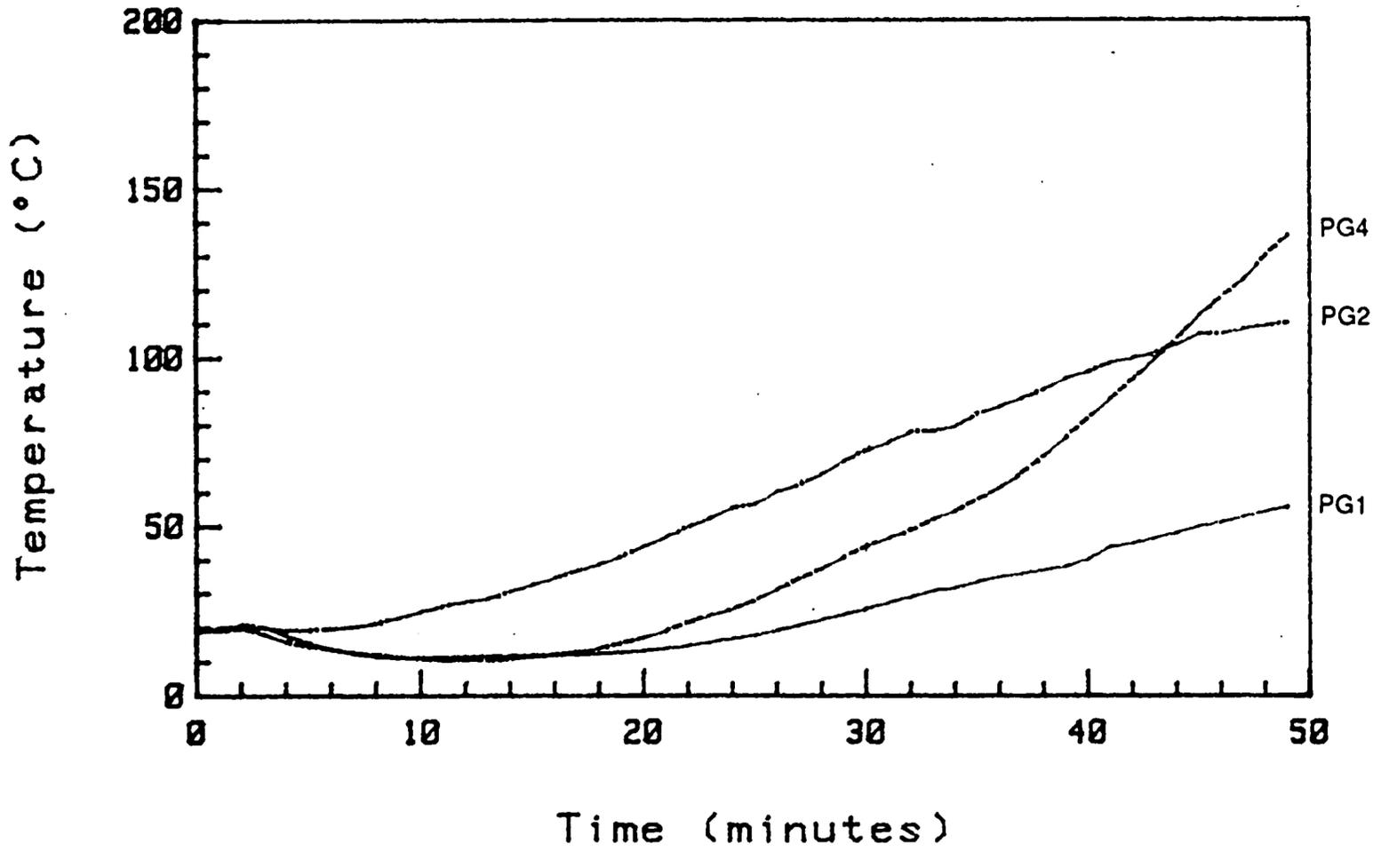
Figure 13a: Temperatures on beam surface beneath gussets, test FS1.
