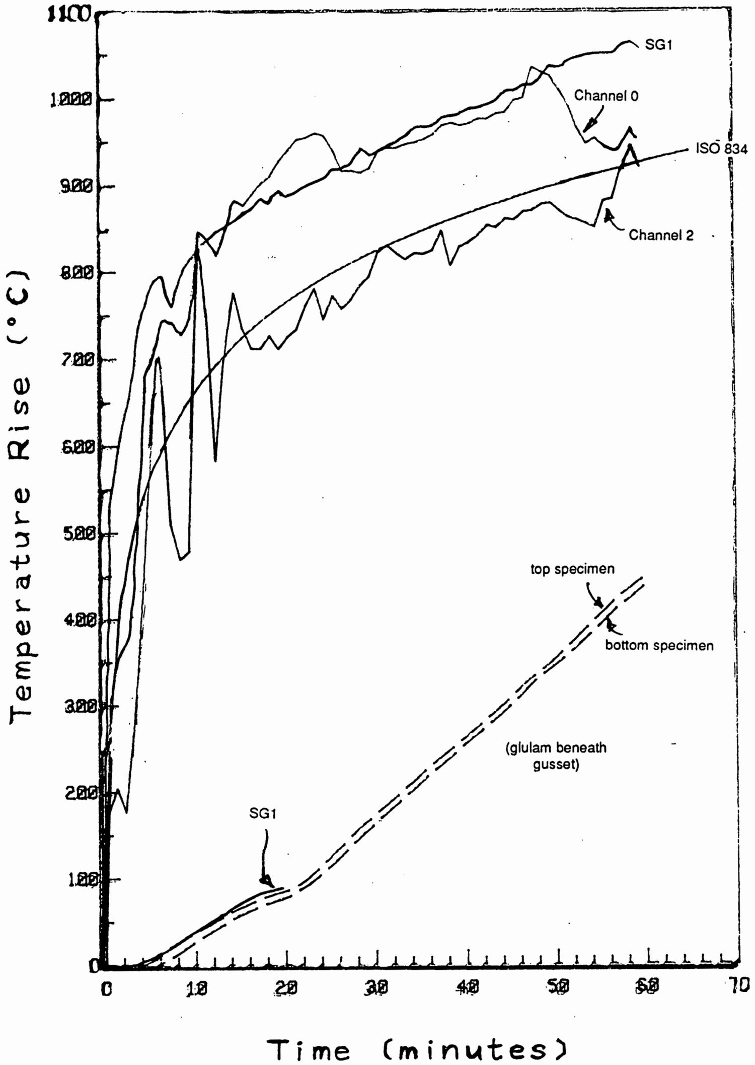
Figure 25b: Temperatures of steel specimens - Test P2.
