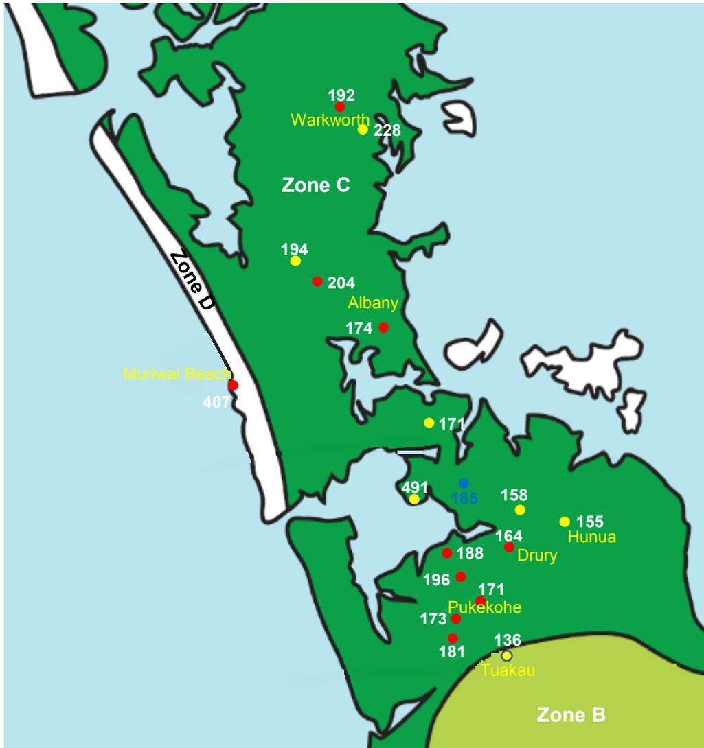
**Figure 3. Schematic showing atmospheric corrosion rate of mild steel in Auckland region (Yellow dots: sites for the 1<sup>st</sup> part of this research; Red dots: sites for the 2<sup>nd</sup> part of this research; Blue dots: sites for other research during 2013 – 2014)**
