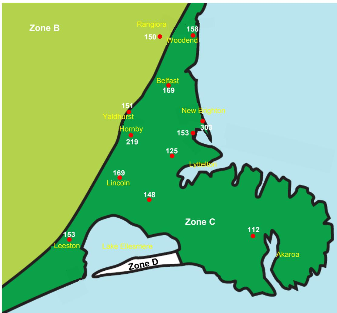
Figure 6. Schematic showing atmospheric corrosion rate of mild steel in Christchurch region
