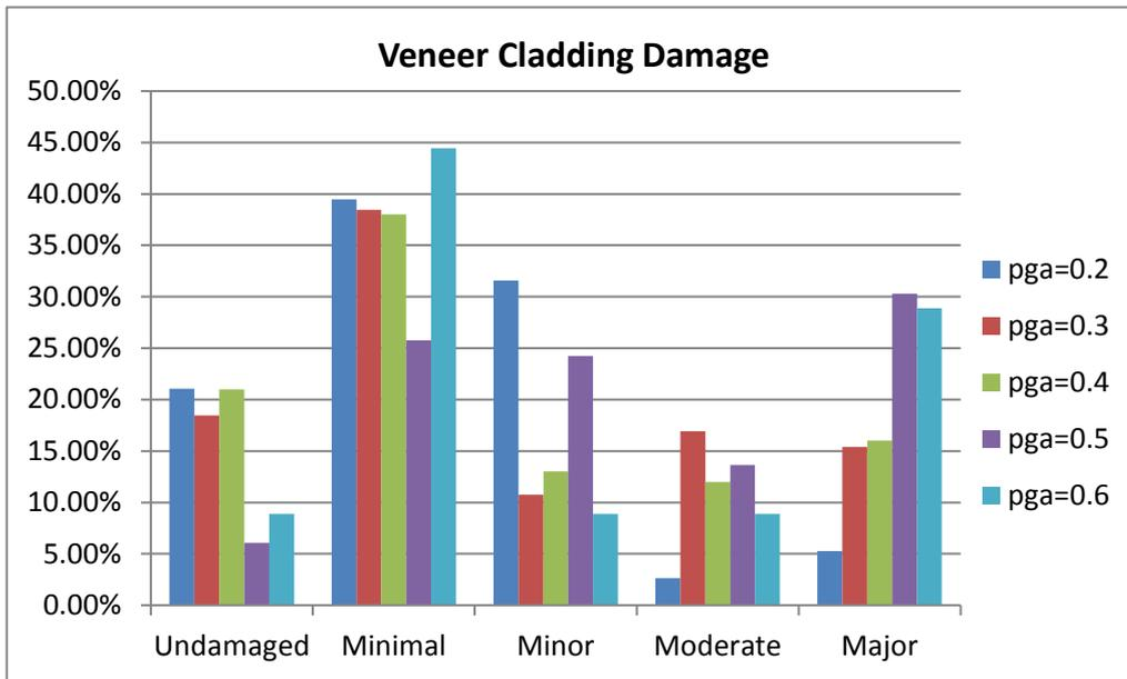
Figure 11. Veneer damage as a function of peak ground acceleration
