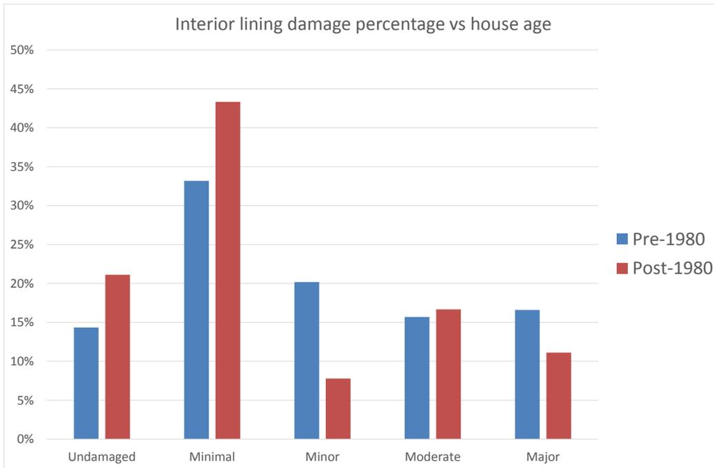
**Figure 17. Comparison of interior lining damage with house age**
