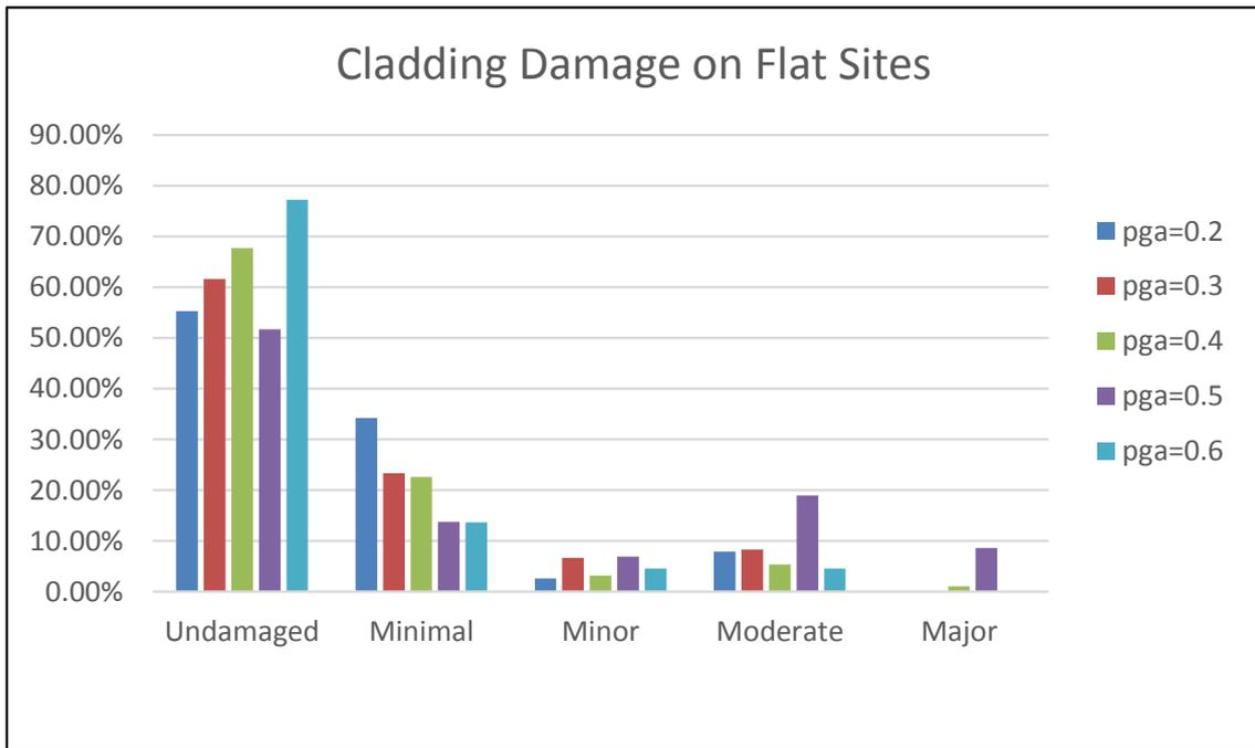
**Figure 22. Veneer cladding damage as a function of PGA for flat sites**
