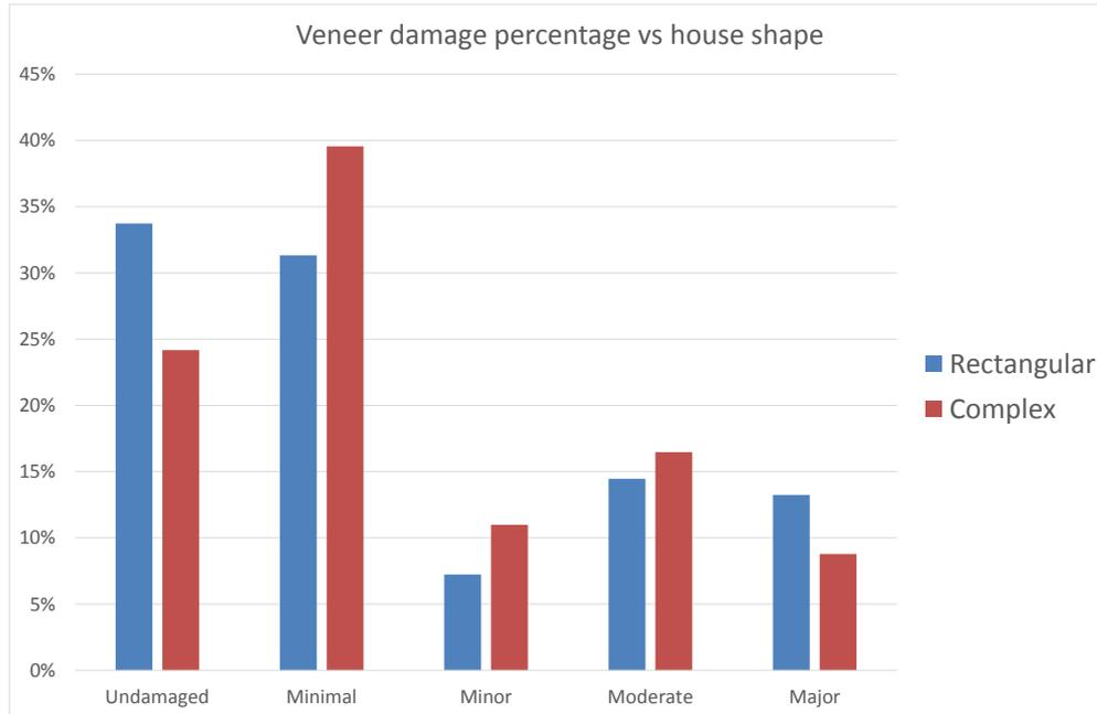
**Figure 14. Veneer damage as a function of house shape**
