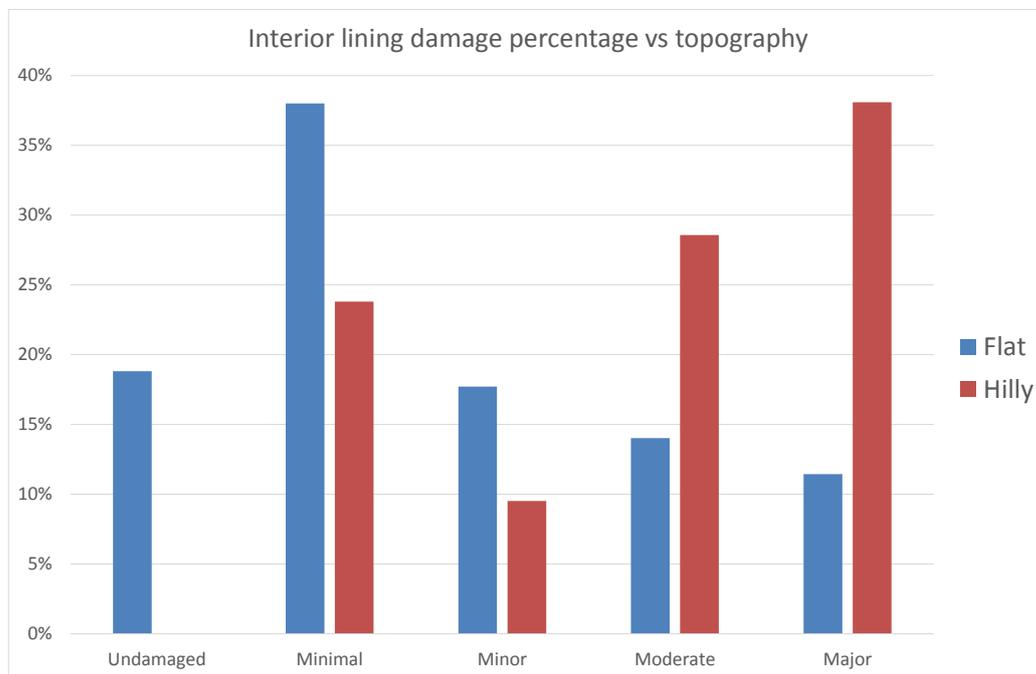
Figure 19. Comparison of interior lining damage against topography
