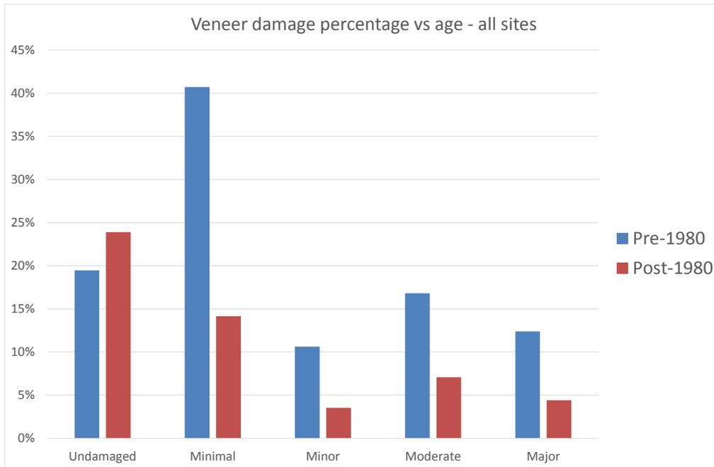
**Figure 12. Veneer damage as a function of house age (all ground conditions)**
