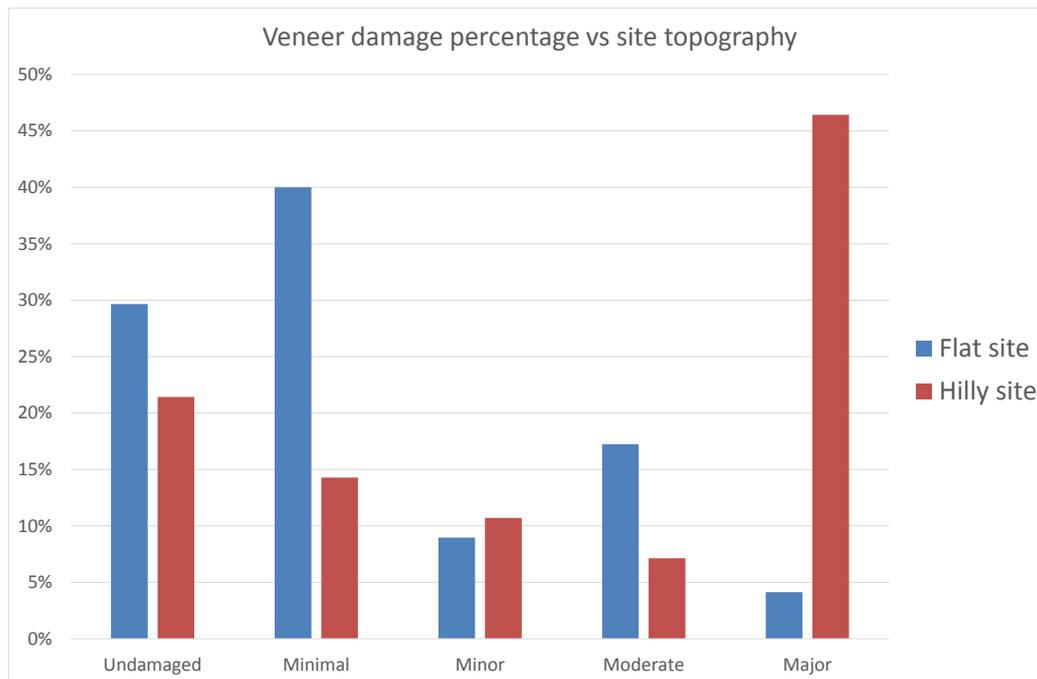
Figure 15. Veneer damage as a function of site topography
