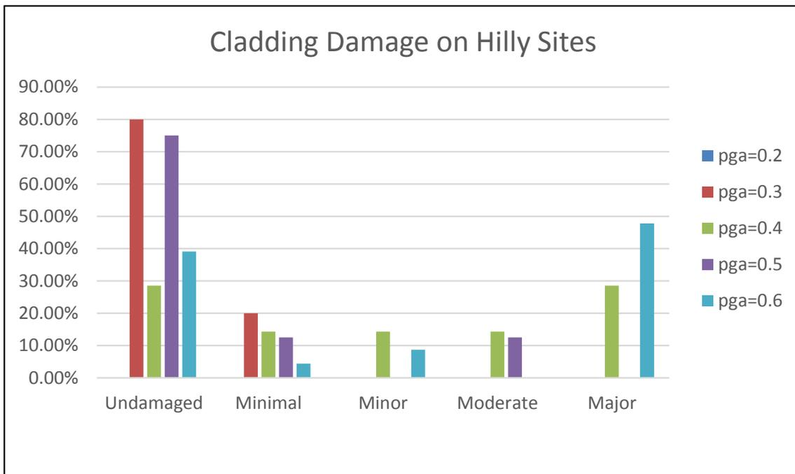
**Figure 23. Veneer cladding damage as a function of PGA for hilly sites**
