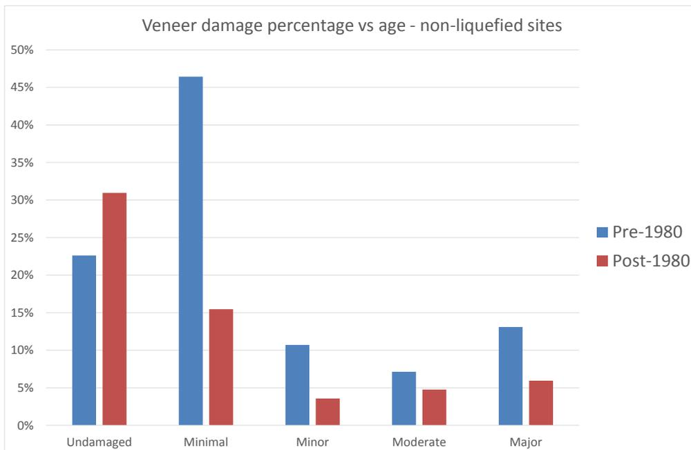
**Figure 13. Veneer damage as a function of house age (non-liquefied ground)**
