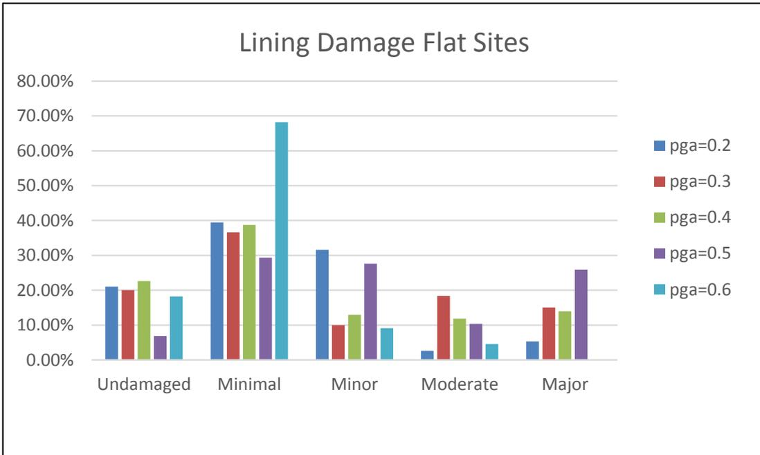
**Figure 20. Lining damage as a function of PGA for flat sites**
