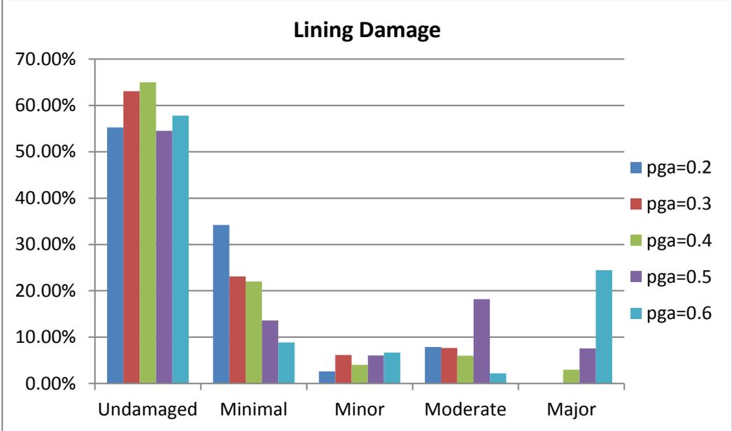
Figure 16. Lining damage as a function of peak ground acceleration
