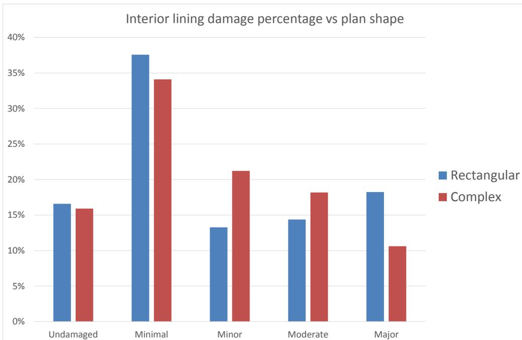
**Figure 18. Comparison of interior lining damage against plan shape**
