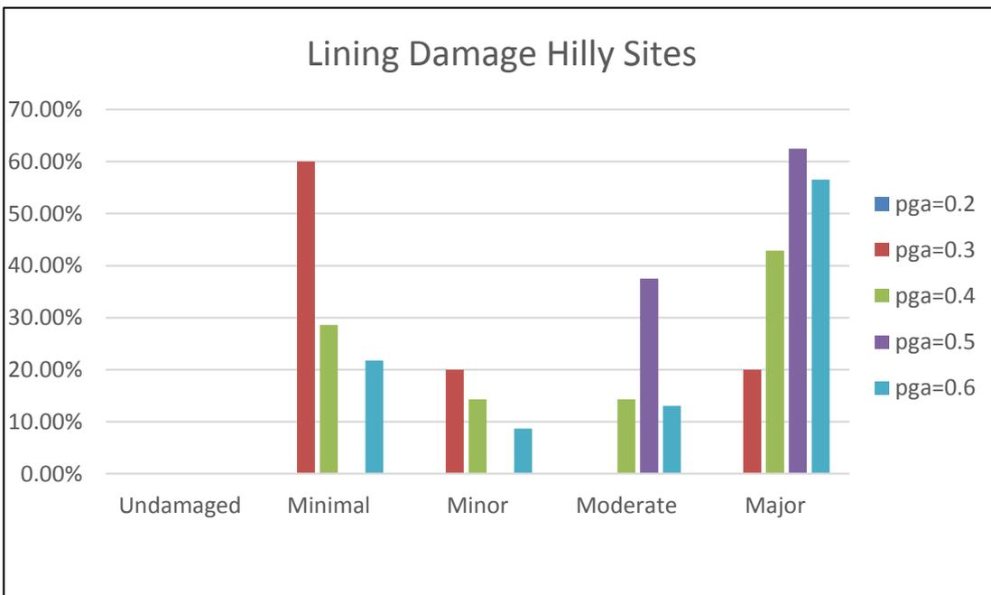
**Figure 21. Lining damage as a function of PGA for hilly sites**
