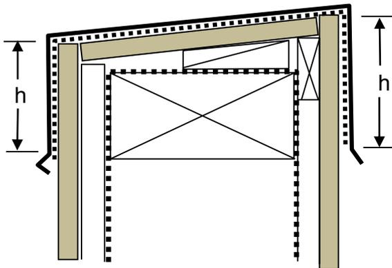
Barge flashing for profiled metal
