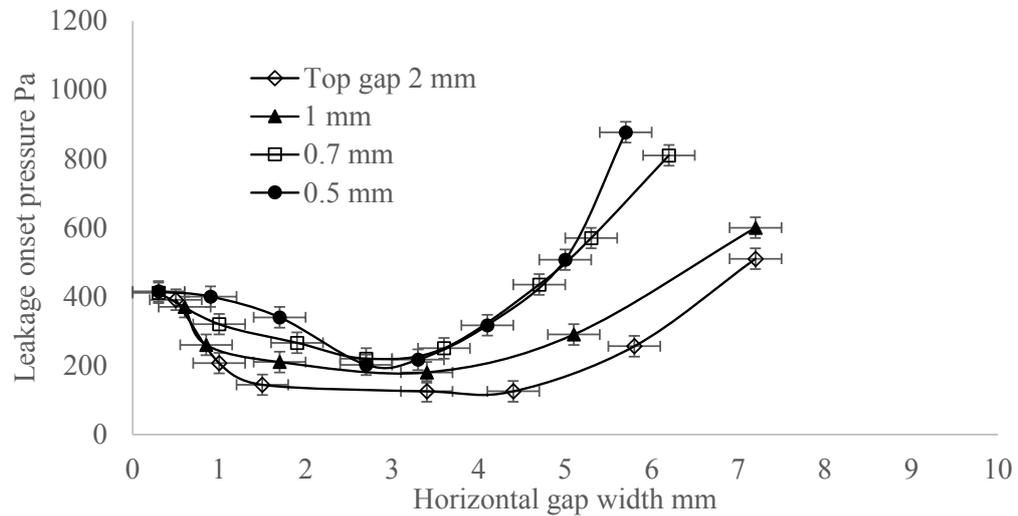
**Figure 7.** Leakage onset pressures for a 35 mm flashing with a plain leg as a function of downturn gap ( $w$ ) and top gap ( $t$ ) dimensions.
