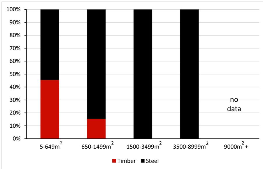
**Figure 2. Roof structure found in surveyed office buildings.**
