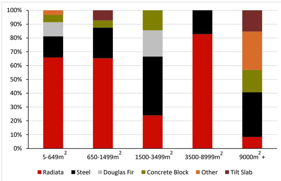
**Figure 6. Wall infill framing found in surveyed office buildings.**
