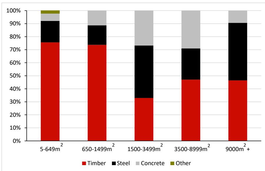
**Figure 5. Partition wall framing found in surveyed office buildings.**
