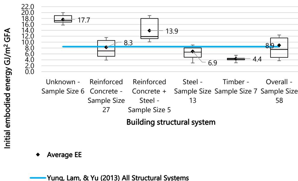
**Figure 8. Summary of embodied energies (EE) of office buildings by structural system (Berg, 2014).**
