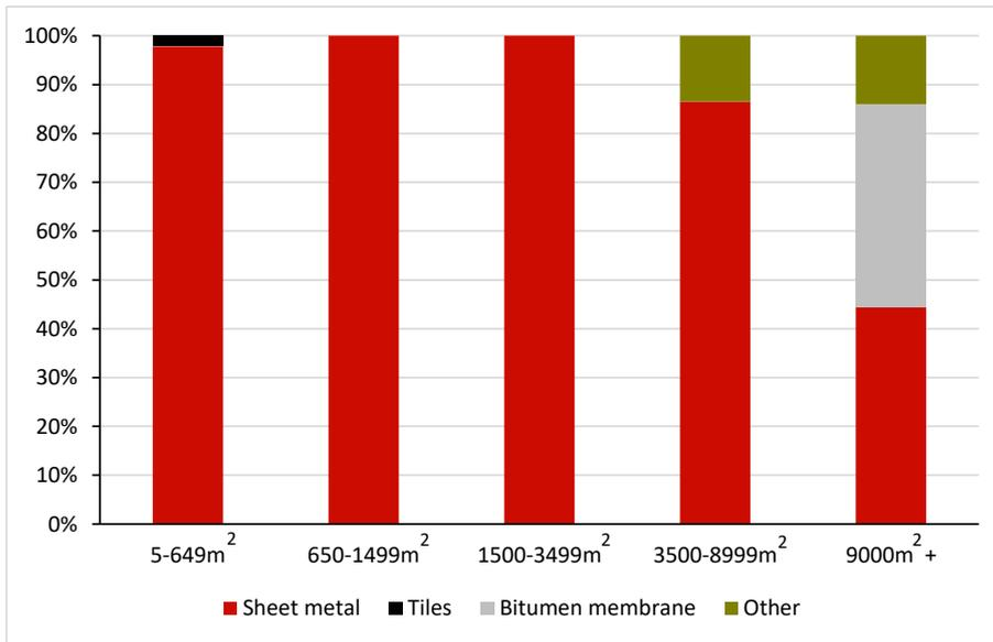
**Figure 4. Roof claddings found in surveyed office buildings.**
