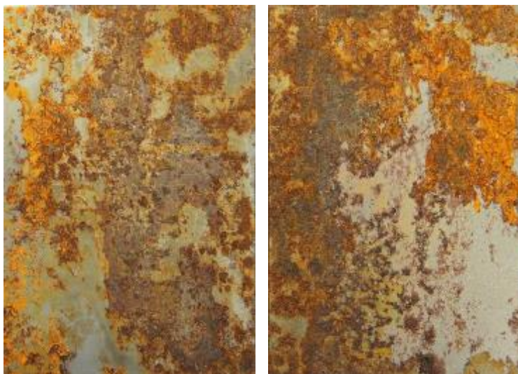
Figure 23. Surface morphology of sandwiched mild steel sample installed close to the vent-1 location in the subfloor of house 7.
