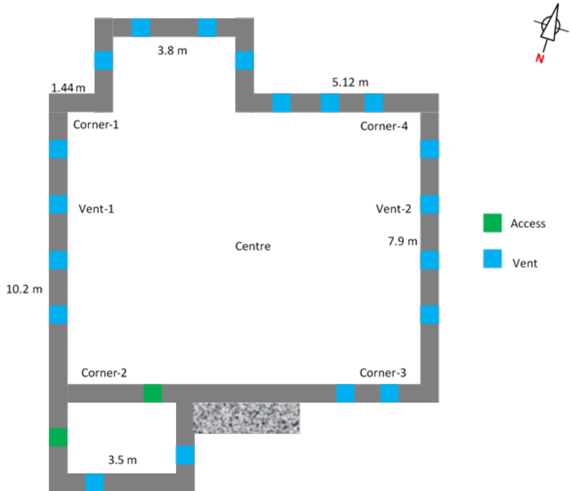
Figure 69. Dimensions of subfloor and sample arrangement of house 4.
