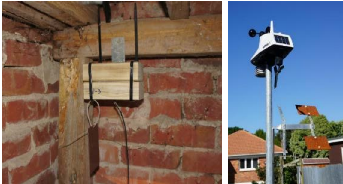
Figure 3. A typical sample set for subfloor (left) and open atmosphere (right) corrosivity measurement.
