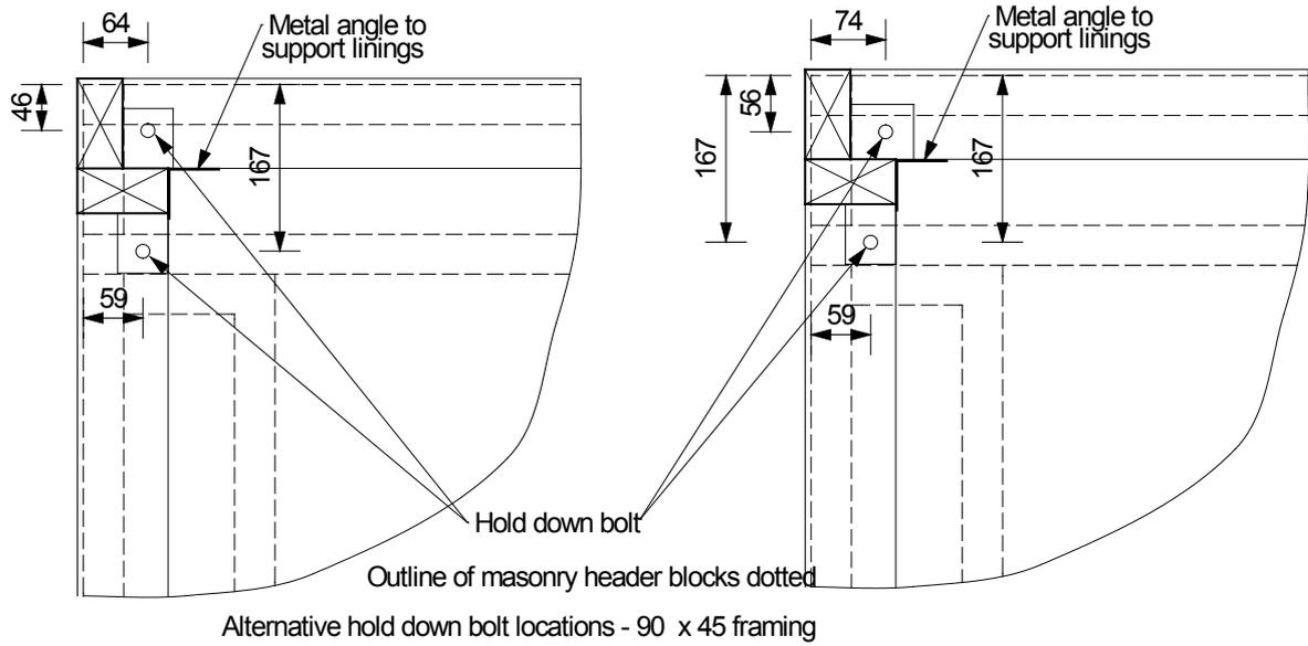
**Figure 3. Layout of reduced wall framing at a foundation corner showing hold-down bolt locations – note that the upper hold-down bracket is either fixed to the stud in the lower wall (left diagram) or the stud in the upper wall (right diagram).**
