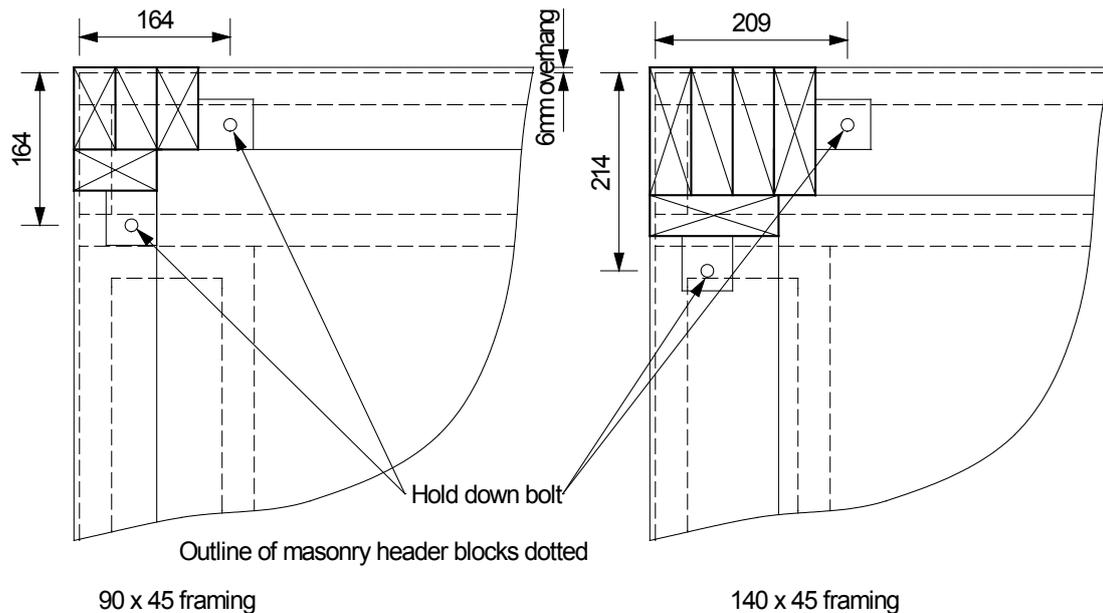
**Figure 2. Layout of traditional wall framing at a foundation corner showing hold-down bolt locations.**
