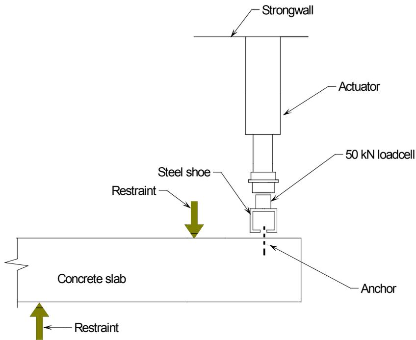
**Figure 6. Plan view of the test set-up.**
