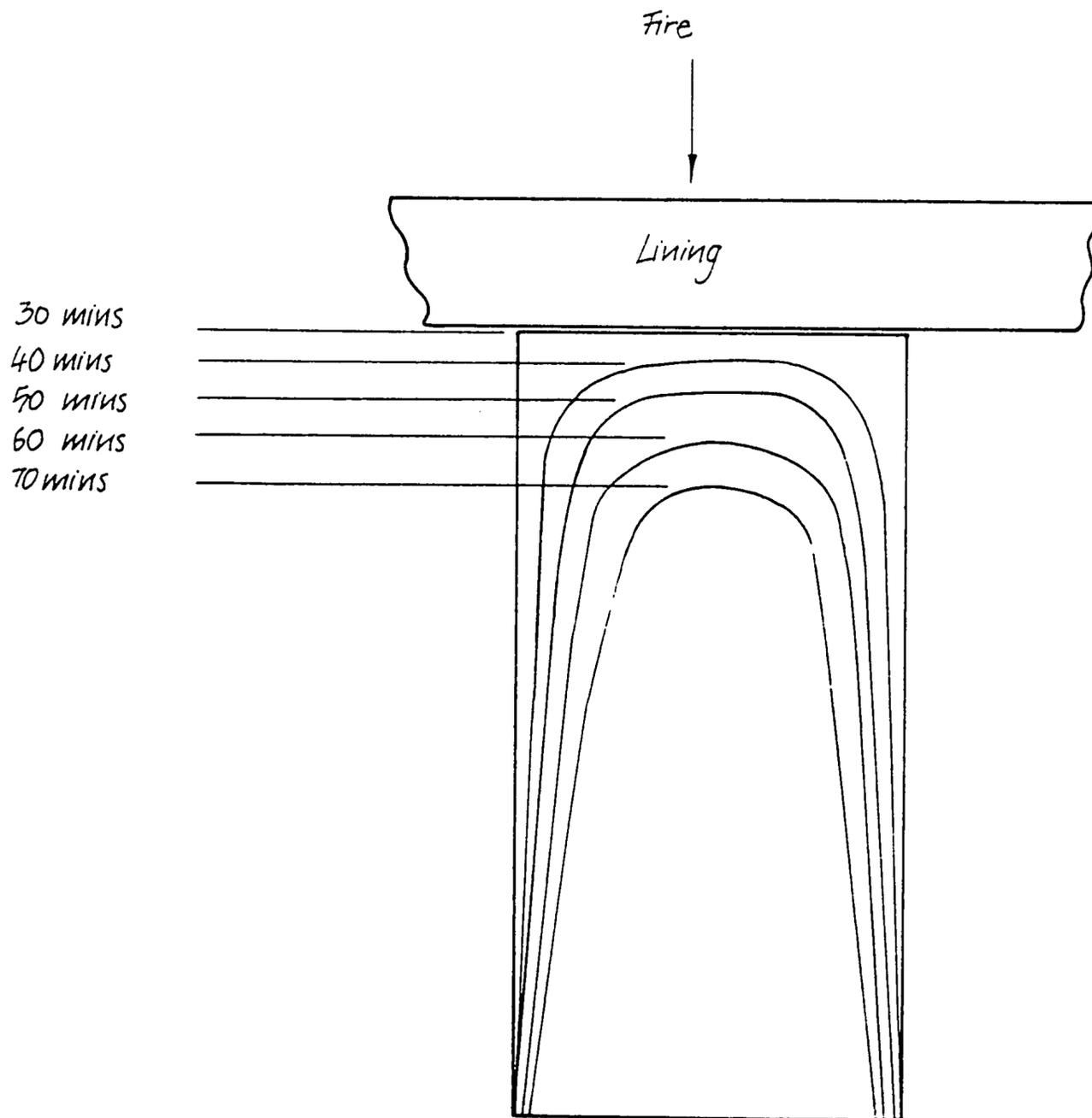
Figure 12: Typical Char Profiles at 10 Minute Intervals on a 100 x 50 Stud
