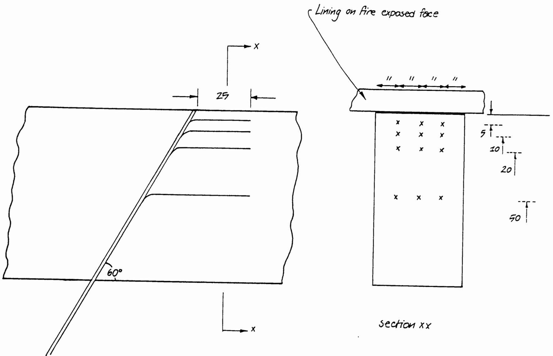
12 sheath thermocouples marked "x" were embedded into a sectioned stud (dummy) as shown at the depths indicated and the stud was then glued back together and installed in wall as shown in Figure 3.
