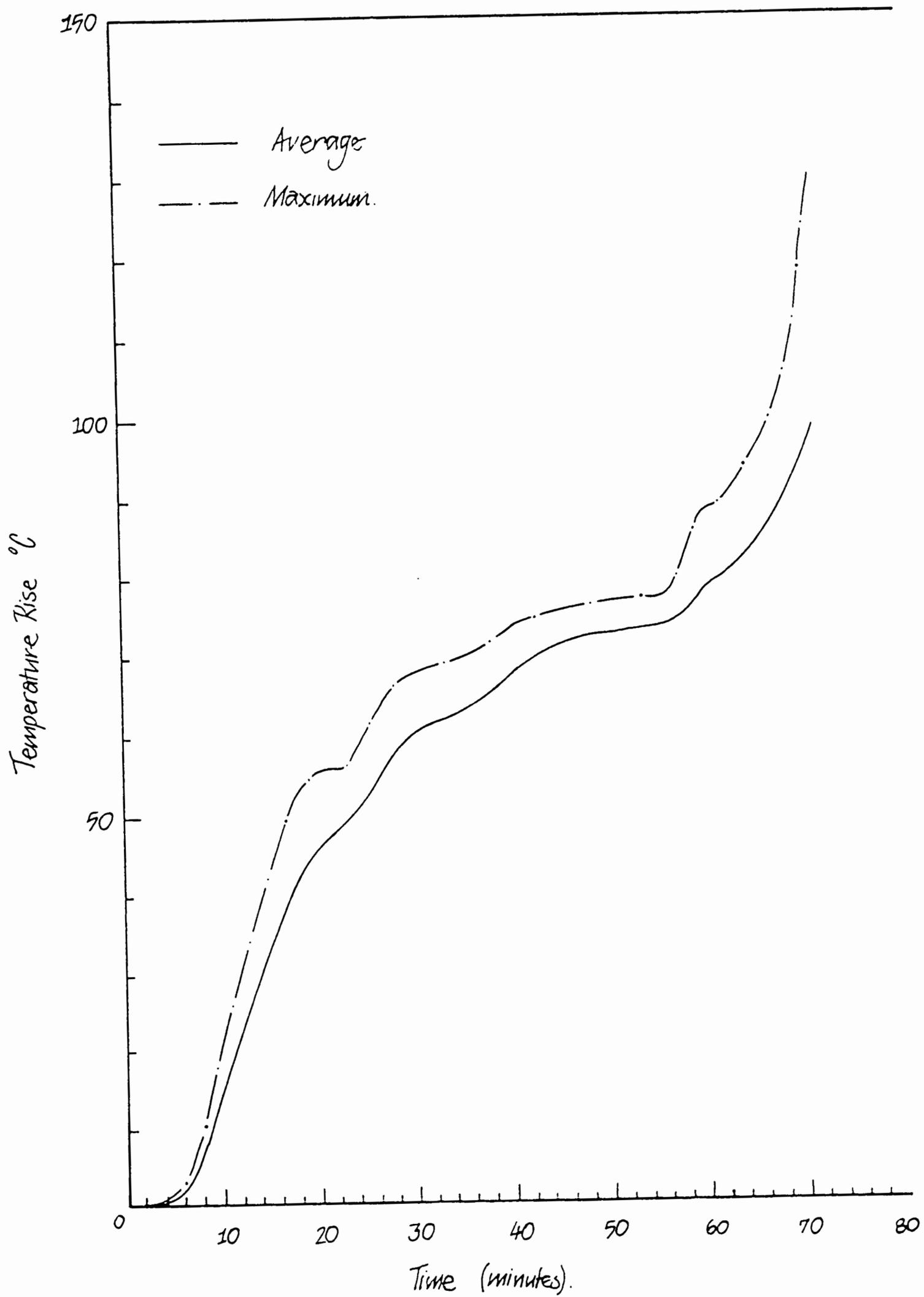
Figure 10: Typical Temperature Rise of Non-Exposed Face of Non-Exposed Plasterboard Lining, Insulation Criterion of Failure
