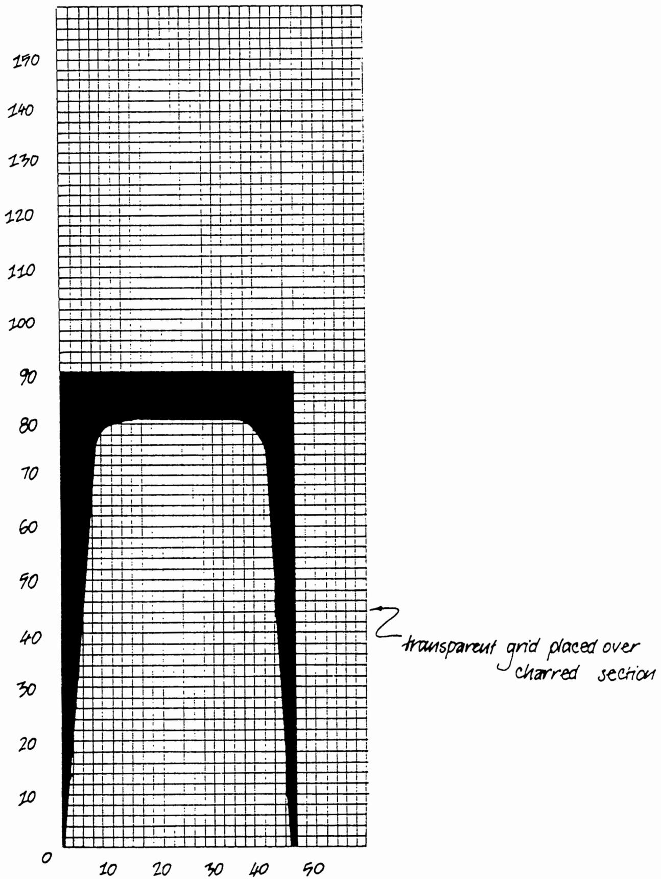
Figure 24: Method of Calculating A, I, C for Residual Stud Cross-Section
