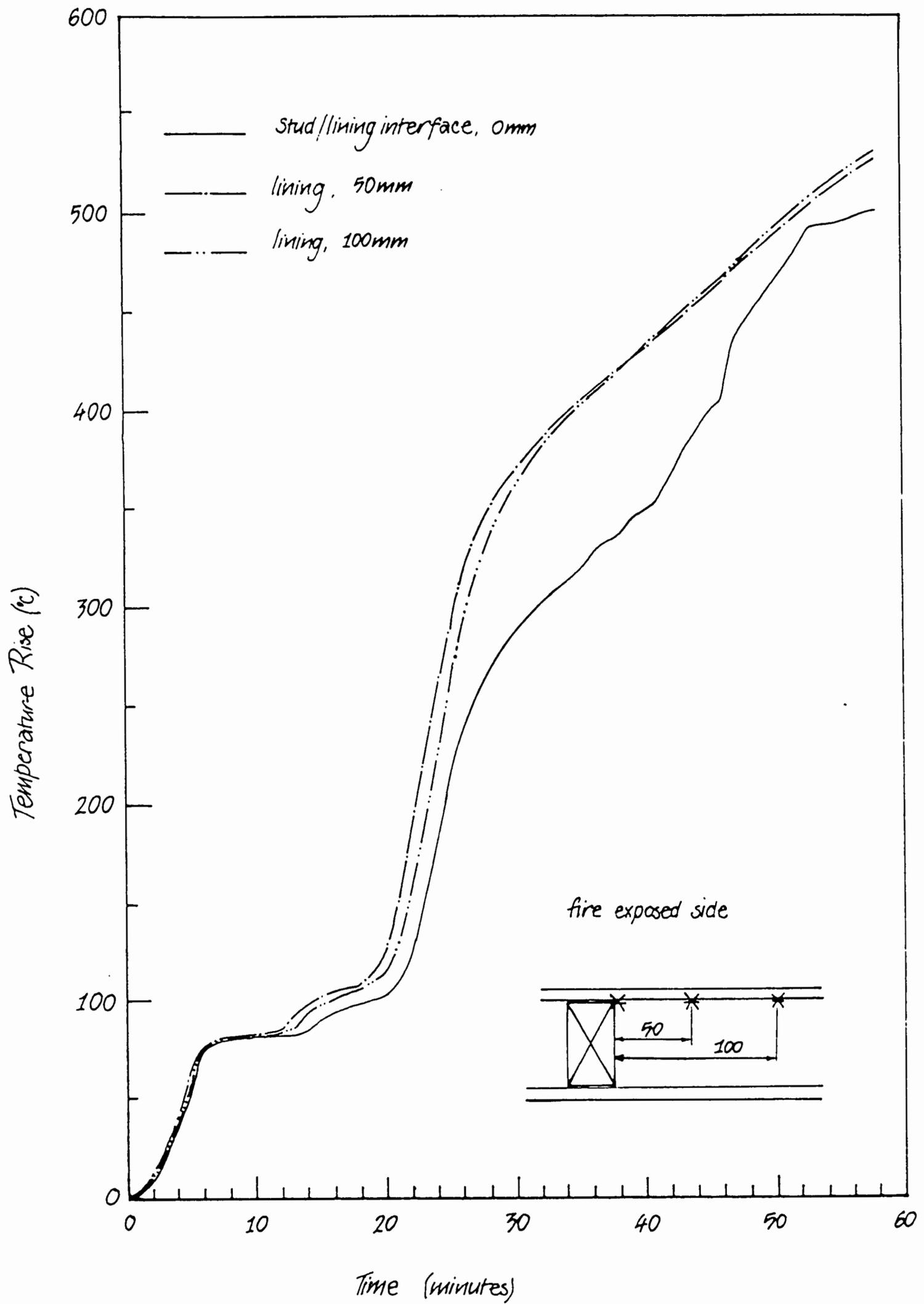
Figure 11: Typical Temperature Rise of Exposed Plasterboard Lining (non-exposed face)
