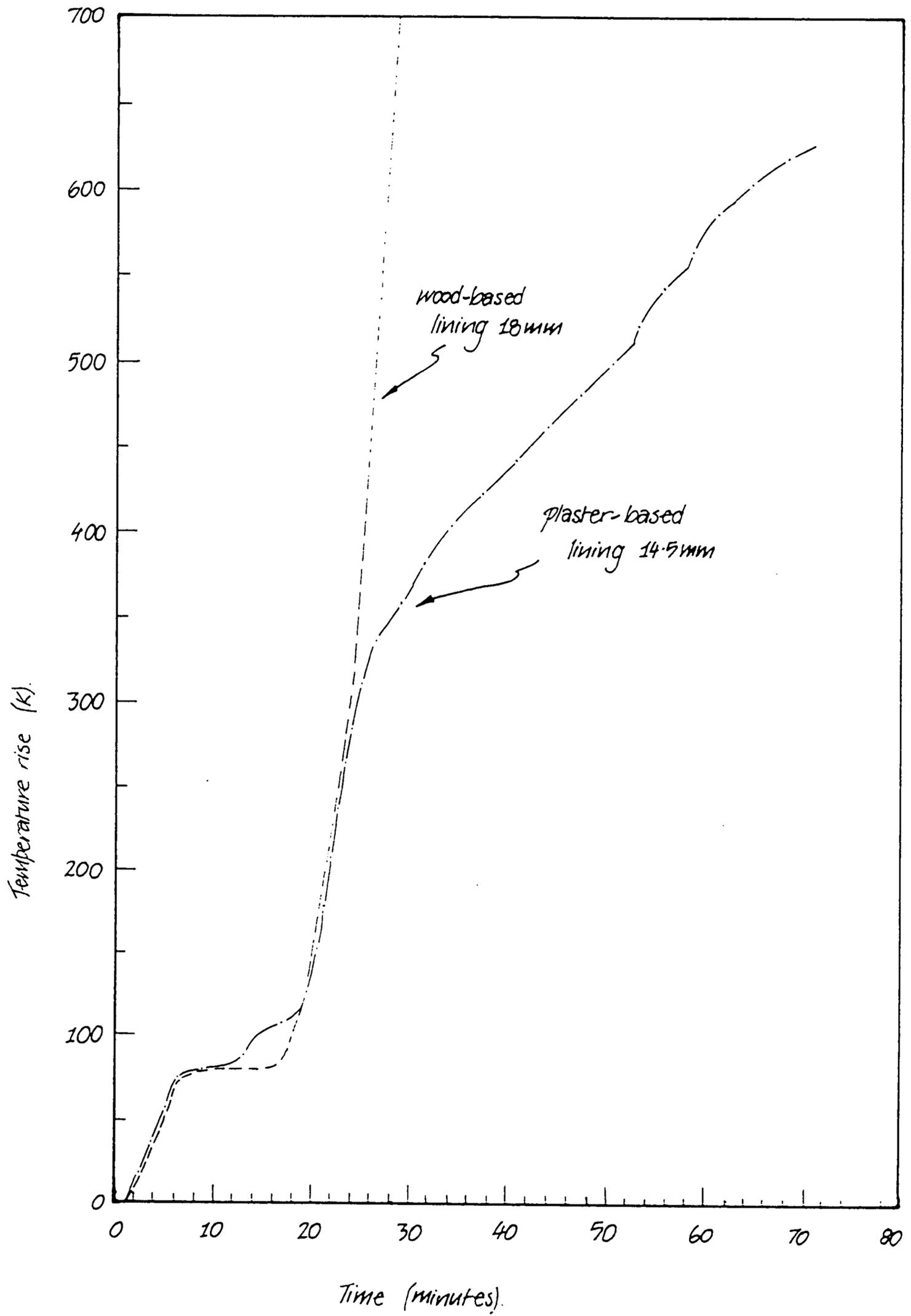
Figure 17: Typical Temperature Rise of Un-Exposed Face of Exposed Lining, for Plaster-Based Linings and Wood-Based Linings
