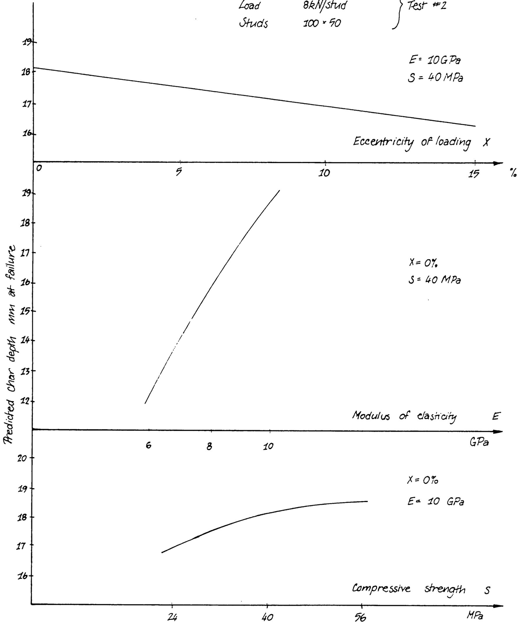
Figure 23: Relative Effects of Variations in Timber Properties
