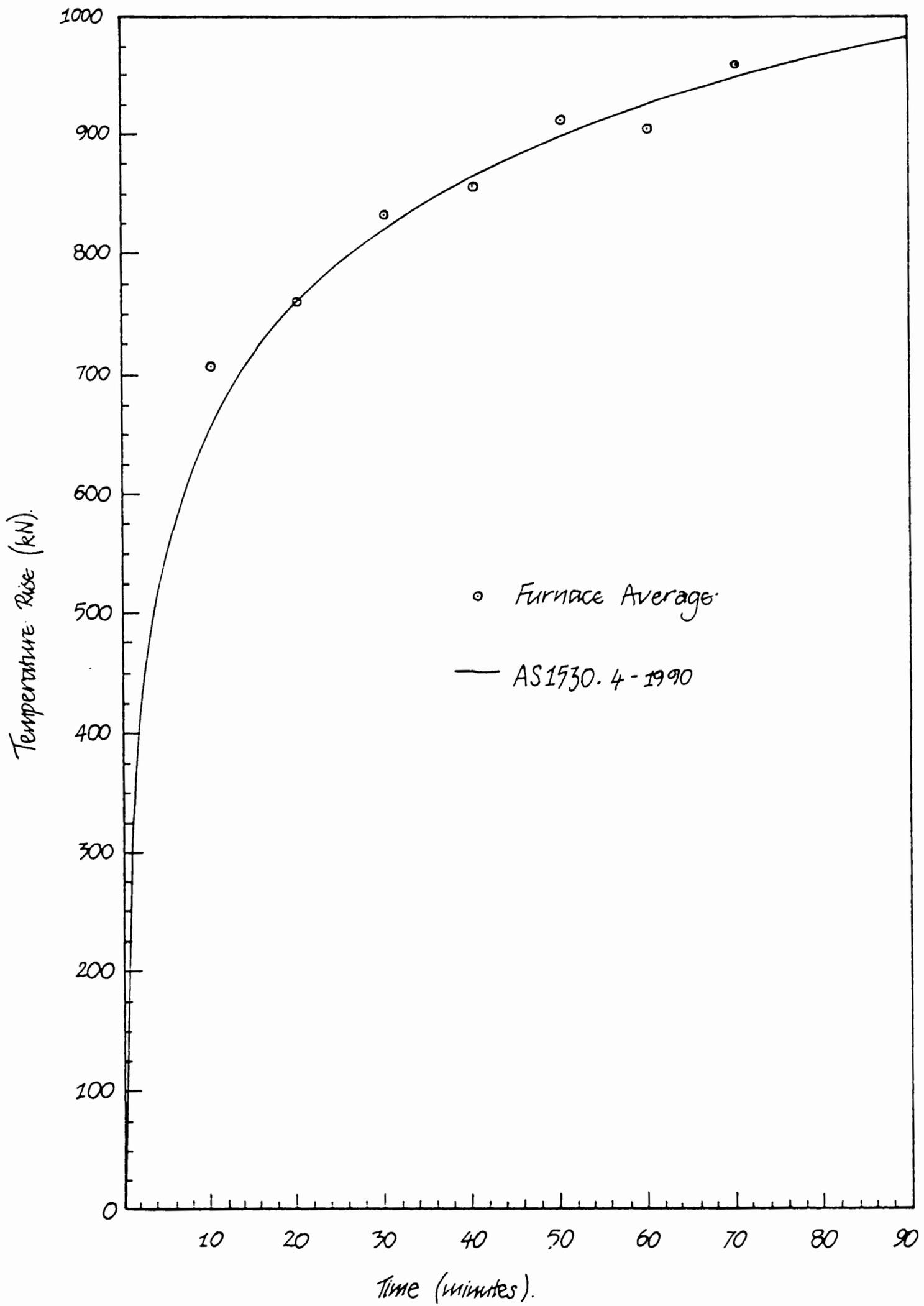
Figure 9: Furnace Temperatures
