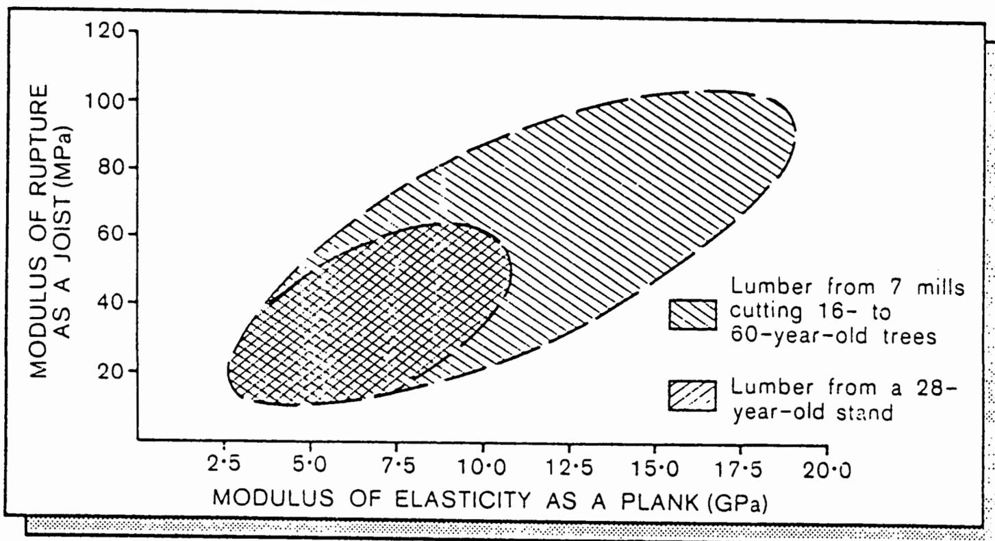
Figure 3: Relationship between Modulus of Rupture and Modulus of Elasticity
