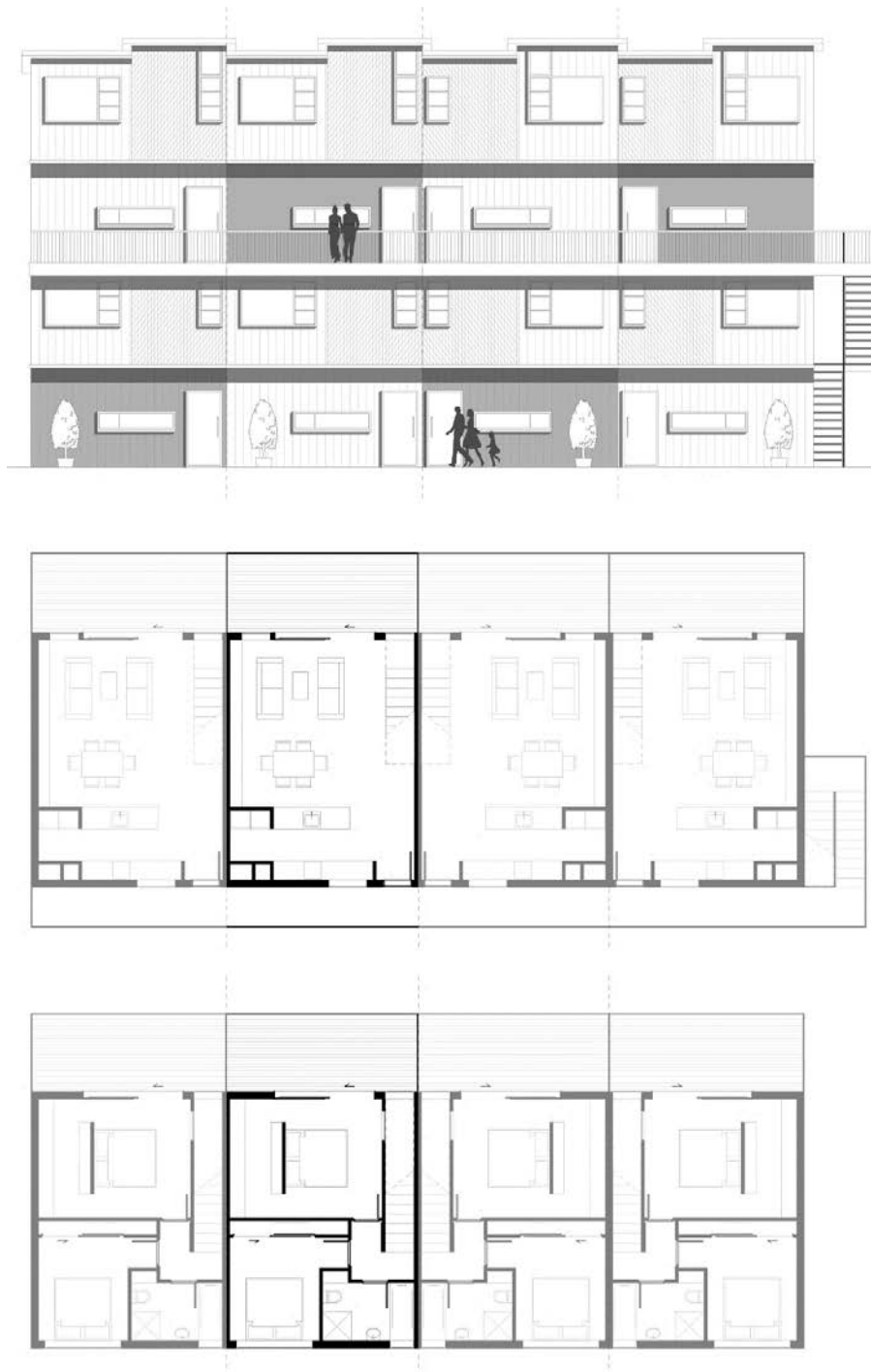
Figure 10. Typical 4-storey terraced house elevation and spatial layout.
