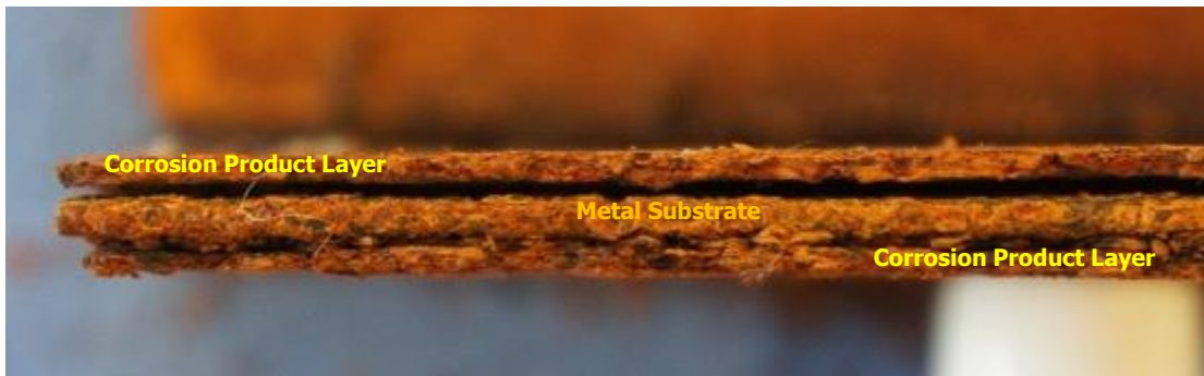
Figure 15. Corrosion products remaining on the mild steel sample exposed at the wastewater treatment plant site for 1 year.
