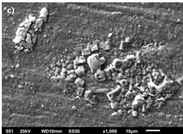
Figure 19. Surface morphology of (a) mild steel, (b) zinc and (c) copper exposed at Judgeford for 1 year.
