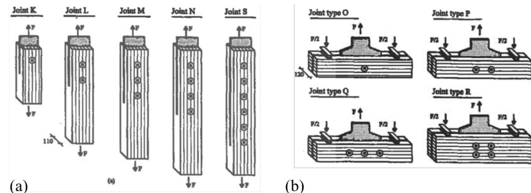
**Figure 16. Glulam-to-steel bolted connections: (a) specimens for parallel-to-grain testing; (b) specimens for perpendicular-to-grain testing.**
