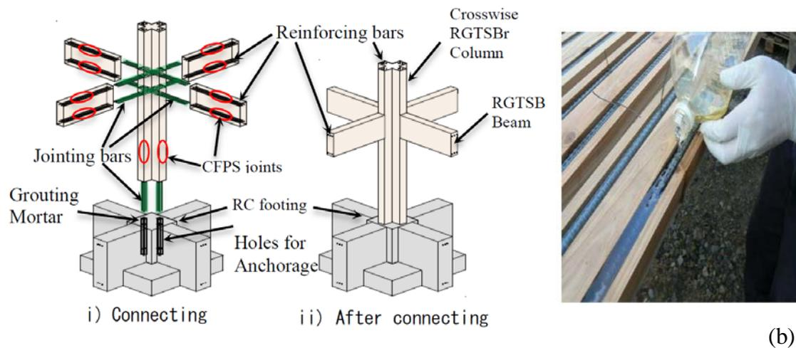
**Figure 4. (a) RGTSB system details; (b) application of adhesive between steel and timber.**
