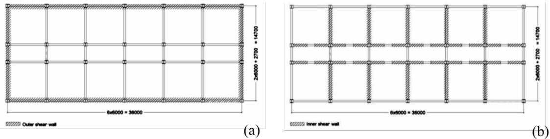
**Figure 12. Steel frames and timber shear walls: (a) external walls; (b) internal walls.**
