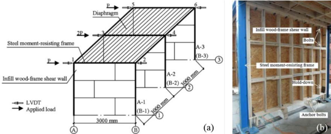
**Figure 1. (a) Specimen dimensions; (b) single hybrid frame type A.**
