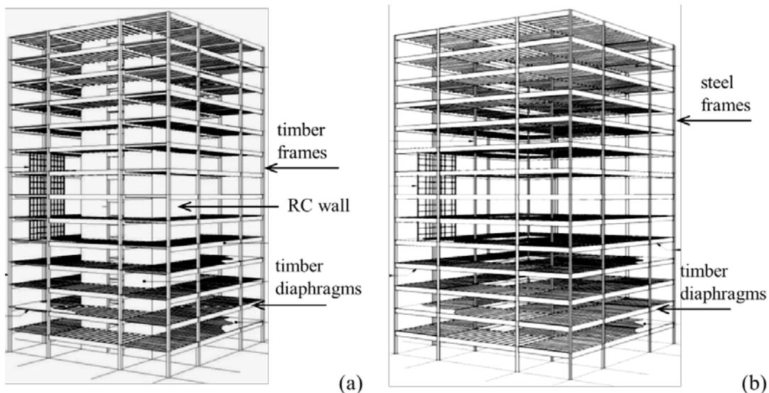
**Figure 27. Hybrid systems proposed by Banks (1999) for 14-storey buildings: (a) case 1: timber gravity frames and flooring plus RC core wall; (b) case 2: steel frame plus timber flooring.**
