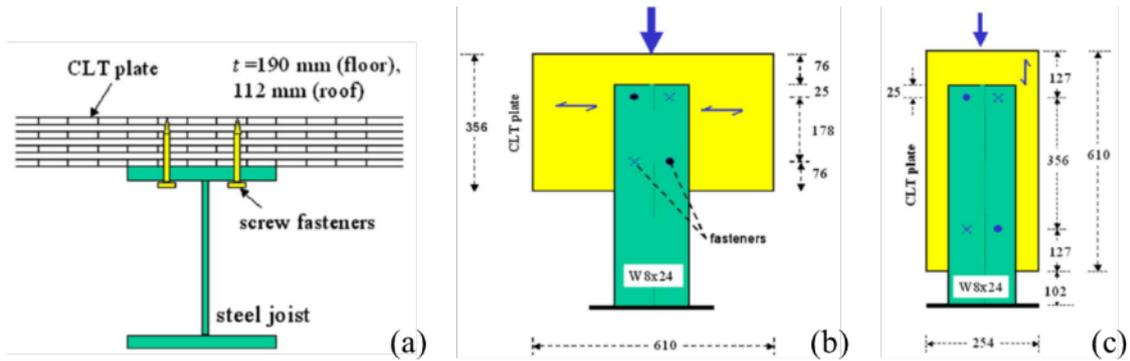
**Figure 17. CLT-to-steel connection: (a) CLT diaphragm over steel beam connected via screws; (b) test set-up parallel to the major axis of CLT plate; (c) test set-up perpendicular to the major axis of CLT plate.**
