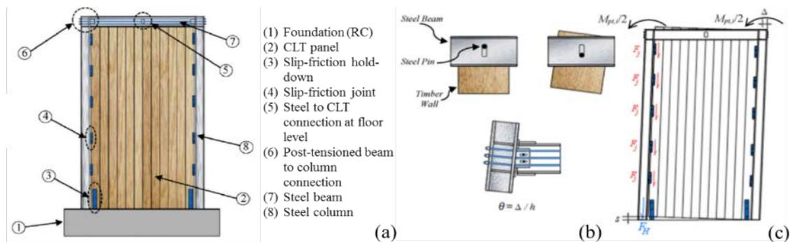
**Figure 14. CLT and steel rocking wall: (a) components; (b) connection details; (c) wall lateral mechanism.**
