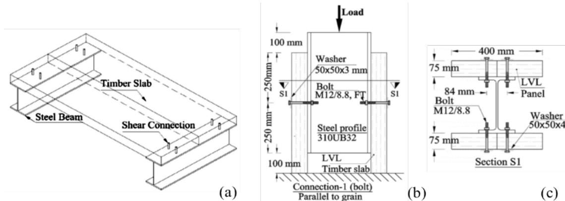
**Figure 19. LVL-to-steel connections: (a) concept for applicability; (b) example of test set-up; (c) cross-section S1 as defined in (b).**
