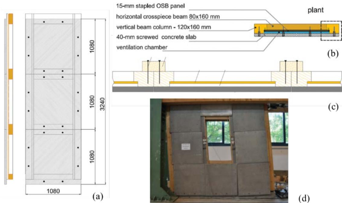
**Figure 3. Timber walls plus RC panels: (a) panel elevation; (b) panel plan view; (c) panel side view; (d) specimen C.**
