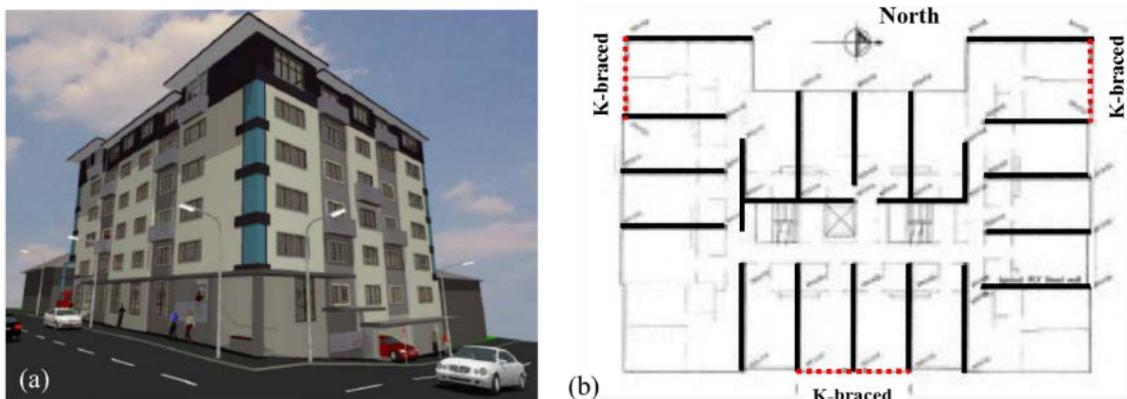
**Figure 22. Hybrid building in Wellington: (a) perspective drawing of the building; (b) super-structure plan layout.**
