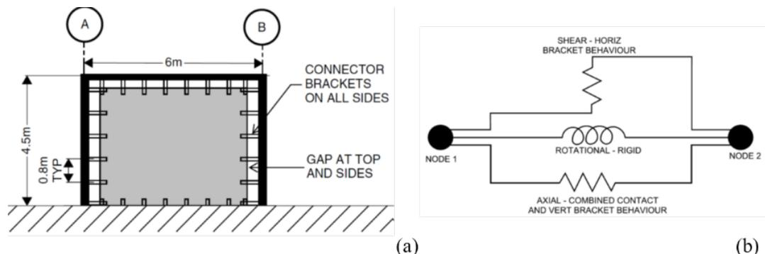
**Figure 13. Steel frame infilled with CLT panel: (a) single-storey, single-span hybrid system; (b) numerical model of the connector brackets.**
