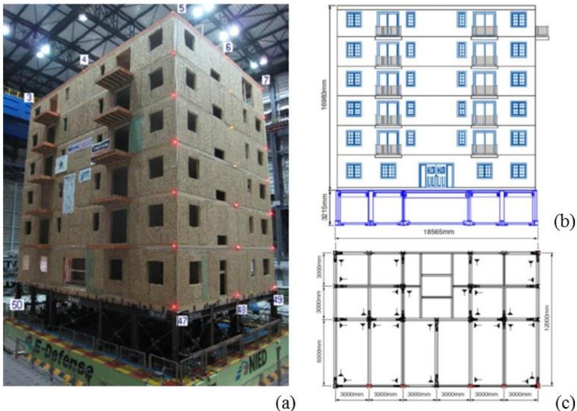
**Figure 5. Full-scale 7-storey shake table testing: (a) Picture taken from the north-west (orientation defined in (c)); (b) north elevation; (c) ground floor plan view.**
