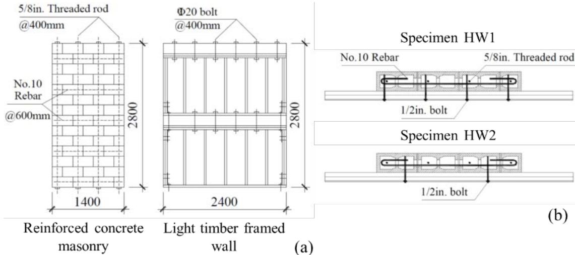
**Figure 2. (a) RCM and LTF walls specimen elevations; (b) plan views of hybrid specimens.**
