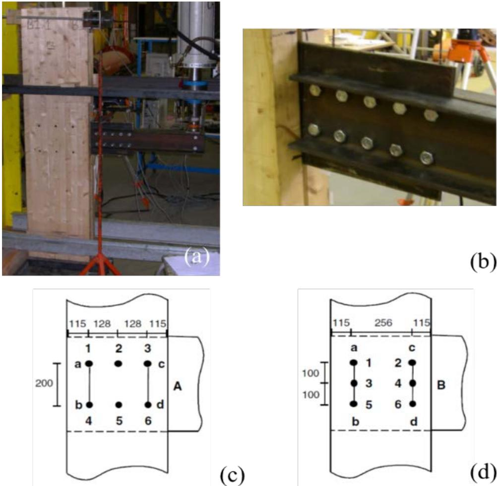
**Figure 20. Steel-to-timber moment-resisting (rigid) connection (a) experimental set-up; (b) steel-plate to steel beam bolted connection; (c) dowel configuration A; (d) dowel configuration B.**
