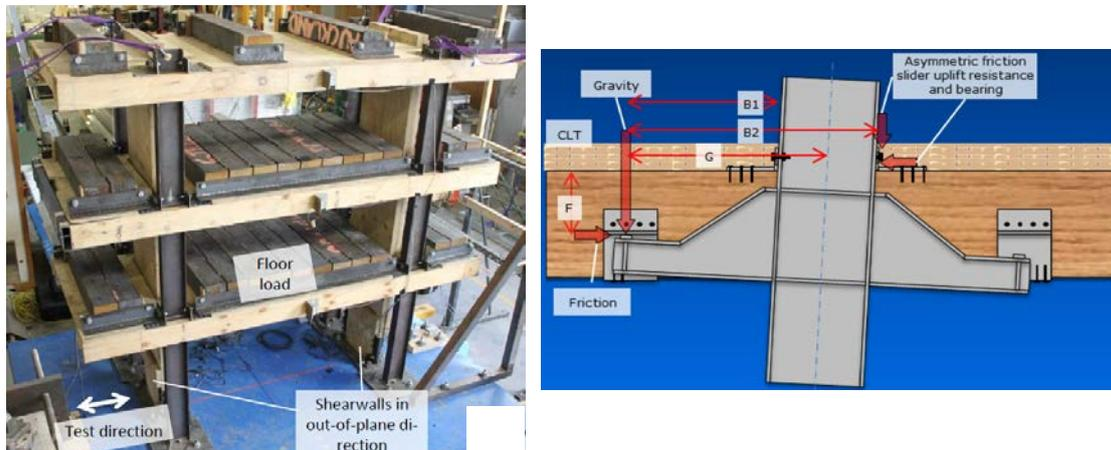
**Figure 6. SHJ shake table testing: (a) picture of the building model; (b) detail of the connection.**
