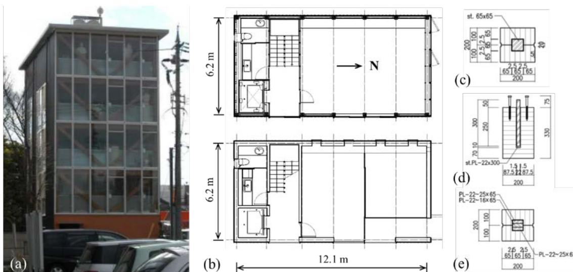
**Figure 23. Hybrid building constructed in Kanazawa, Japan: (a) picture from the northwest; (b) plans of substructure (bottom) and super-structure (top); (c) column cross-section; (d) beam cross-section; (e) brace cross-section.**
