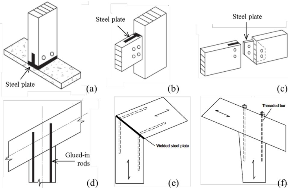
**Figure 15. Concealed traditional timber connections: (a) concrete footing-to-column mechanical; (b) mechanical beam-to-column; (c) mechanical beam-to-beam; (d) column-to-beam glued in rods; (e) beam-to-column glued-in and welded; (f) column-to-beam mechanical with threaded bars.**
