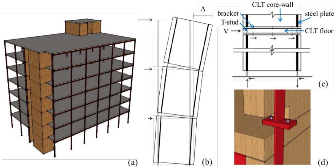
**Figure 11. CLT panels with continuous steel plate connections: (a) hybrid building vision; (b) CLT hybrid wall concept; (c) detail of connection between wall and diaphragm; (d) detail of steel splicing.**
