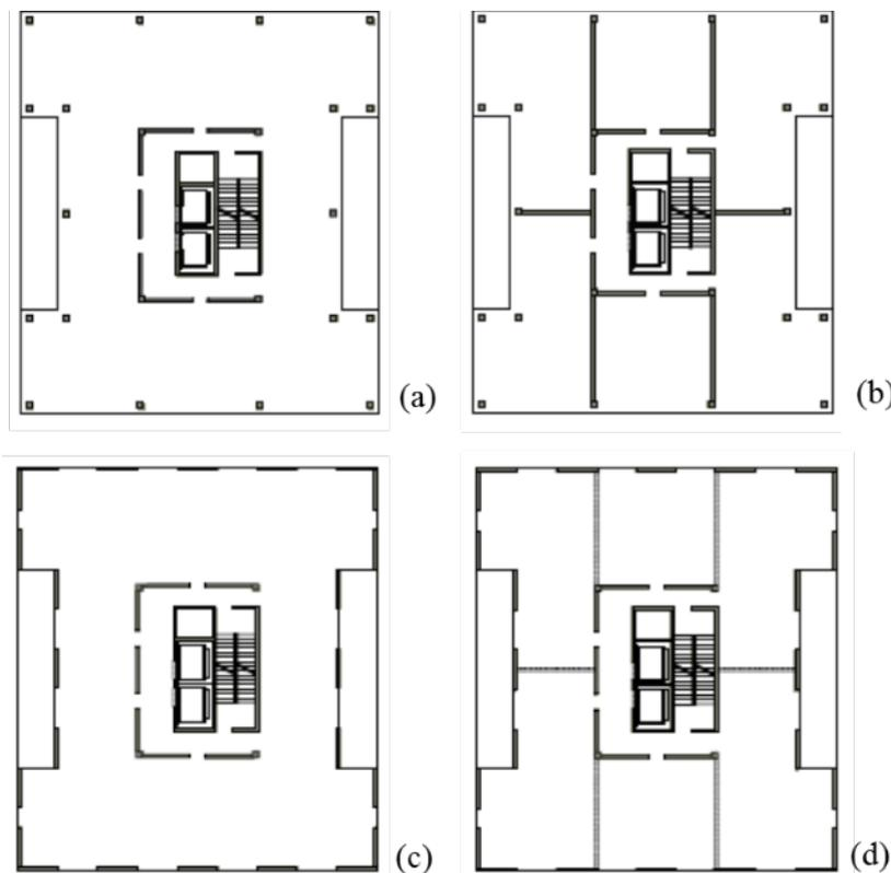
**Figure 10. FFTT system: (a) option 1 – core walls and perimeter frames (up to 12 storeys); (b) option 2 – core and interior walls and perimeter frames (up to 20 storeys); (c) option 3 – core and exterior walls (up to 20 storeys); (d) core, interior and exterior walls (up to 30 storeys).**
