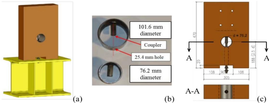
**Figure 18. Steel-tube connection for hybrid structures: (a) test specimen; (b) steel-tube device; (c) detail of connector inside CLT.**
