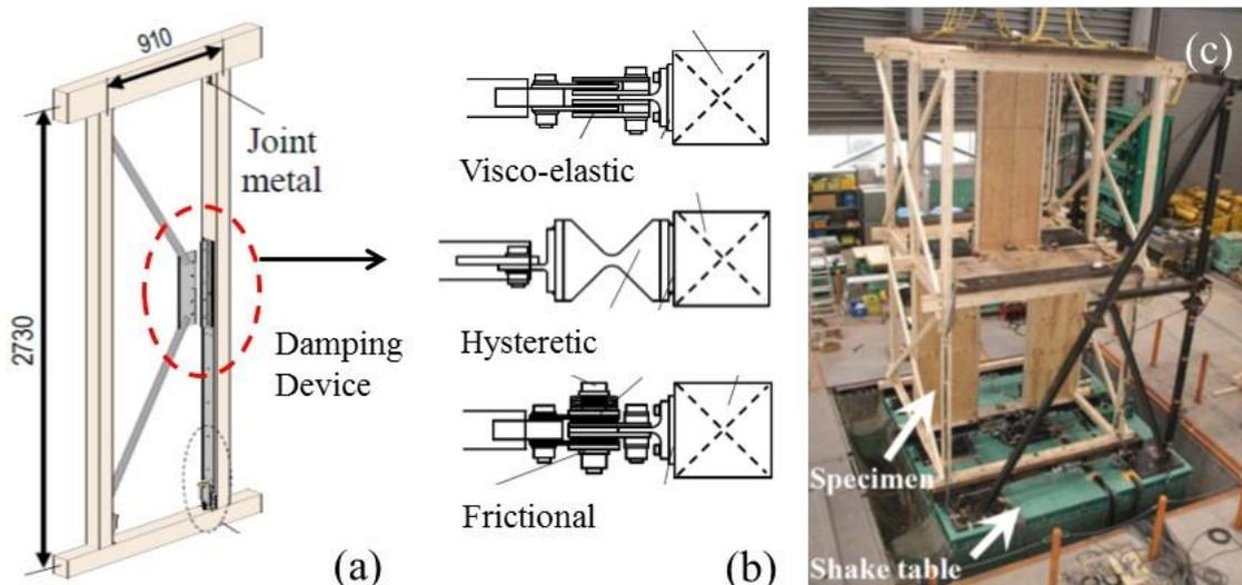
**Figure 7. (a) LTF with damping device and braces; (b) types of damping devices; (c) specimen tested on the shake table.**
