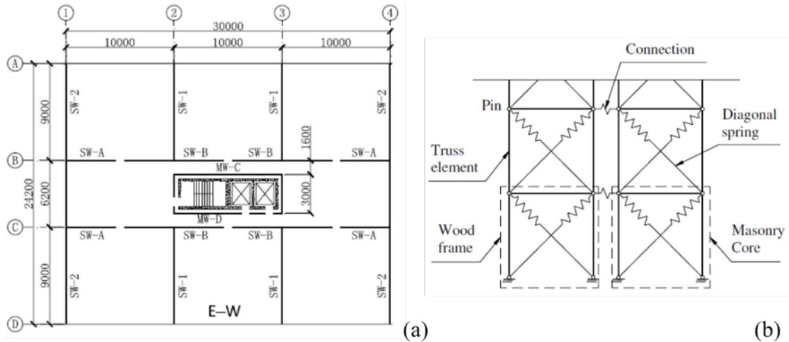
**Figure 9. Numerical investigation on timber-RCM hybrid system: (a) prototype structure layout; (b) model description.**
