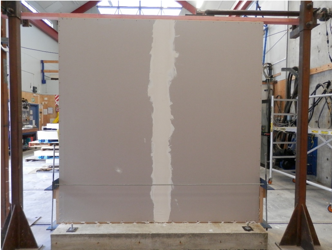
Figure 1. The sheathing (two plasterboard sheets) worked as one plate. Deformation is mainly due to slips.
