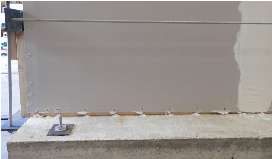
Figure 2. Final appearance after racking on a plasterboard wall of 2.4 m long.
