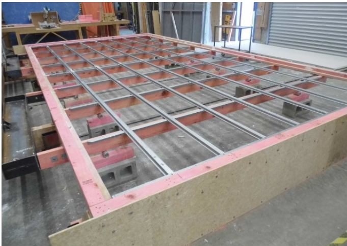
Figure 28. Framing of the full-scale ceiling test specimen.
