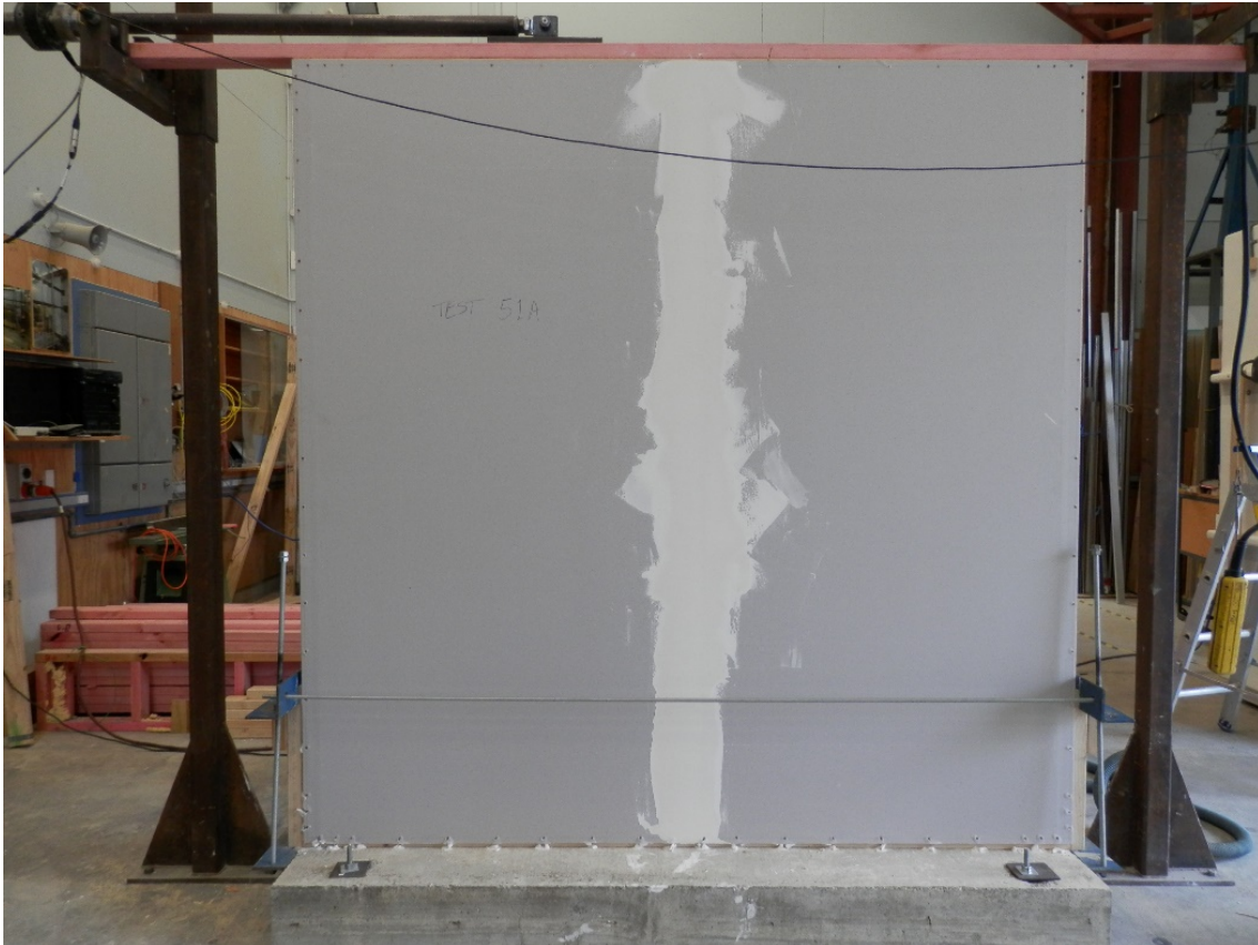
Figure 3. The sheathing (two plasterboard sheets) worked as one plate. Deformation is mainly due to slips.
