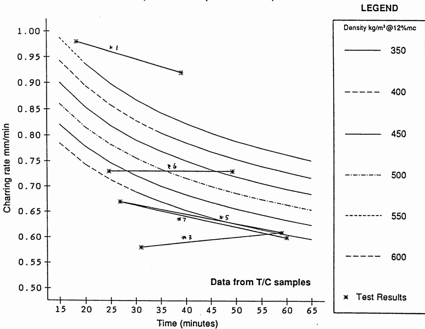
Figure 9 Variation of mean charring rate with exposure time
