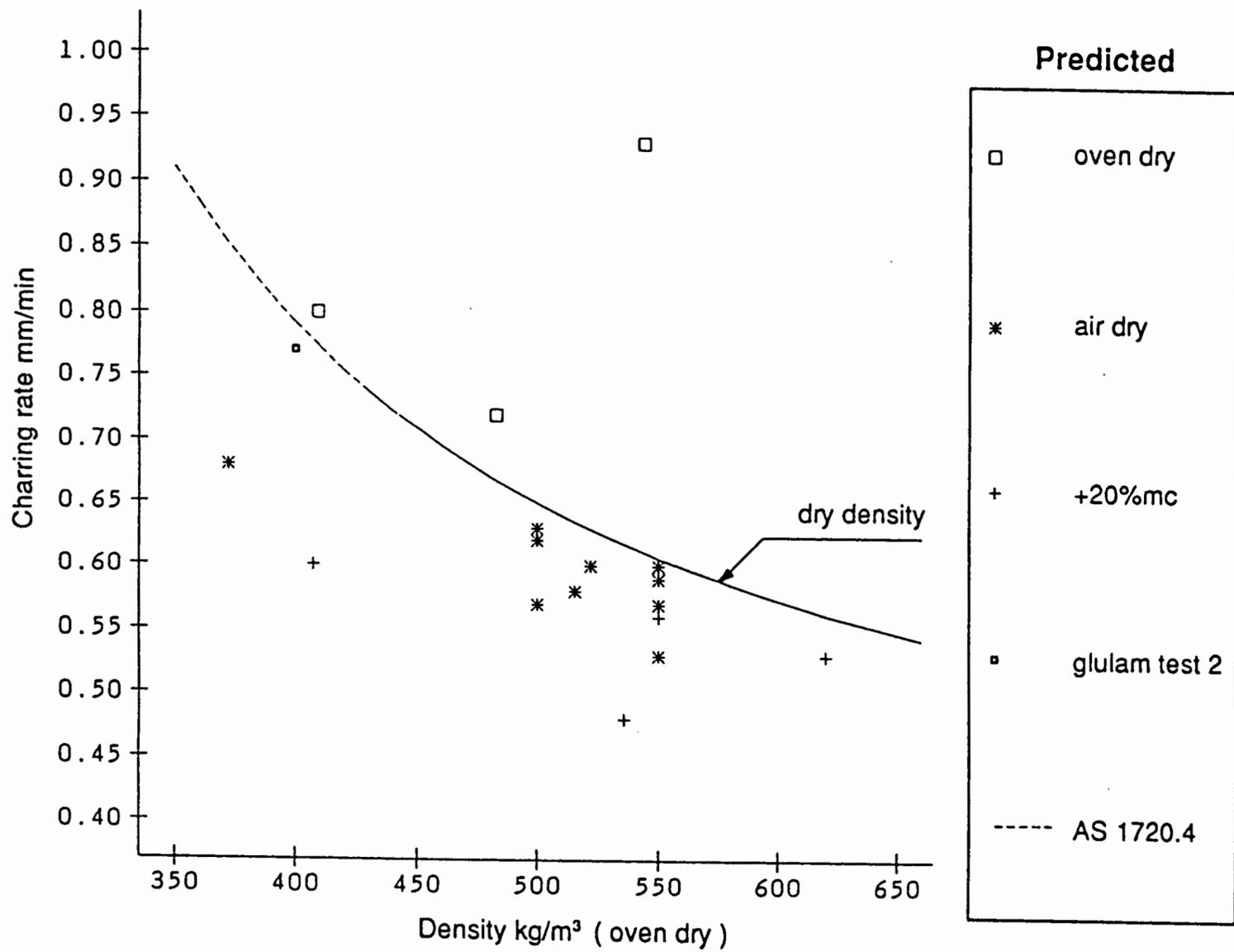
Figure 10 Comparison of test results and AS 1720.4 for 60 minutes
