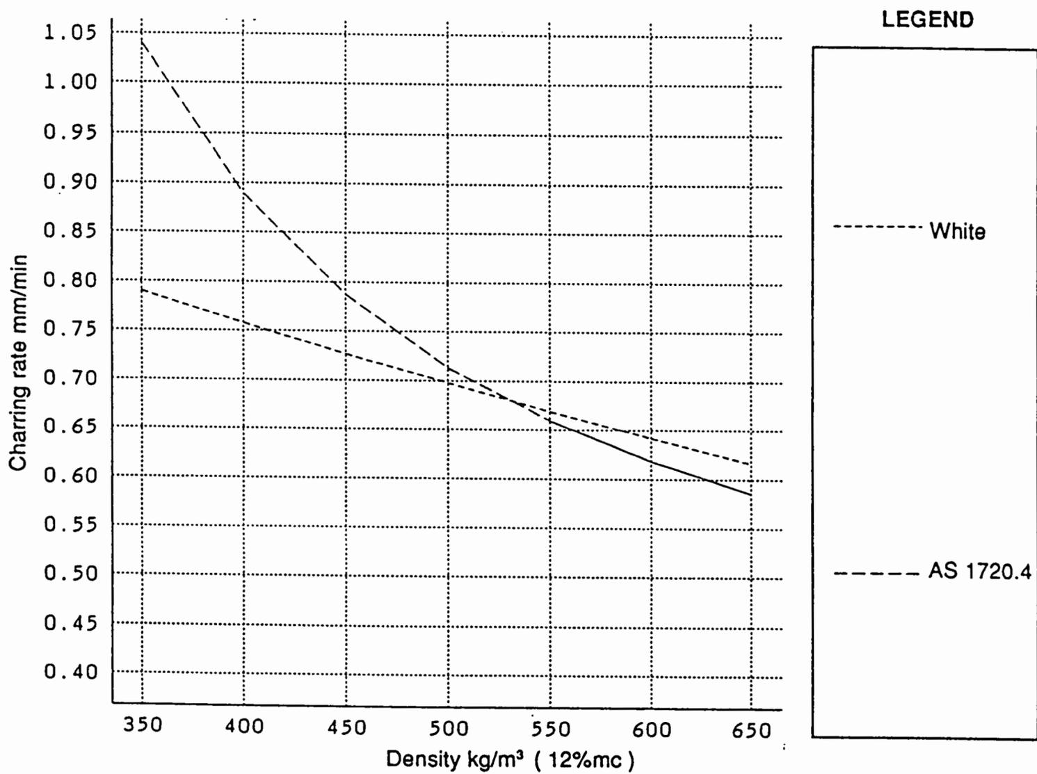
Figure 11 Comparison of charring rate prediction of White's model and AS1720.4
