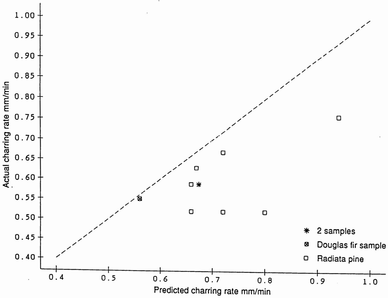
Figure 6.1 Scatter diagram of char rates for 29 minutes exposure
