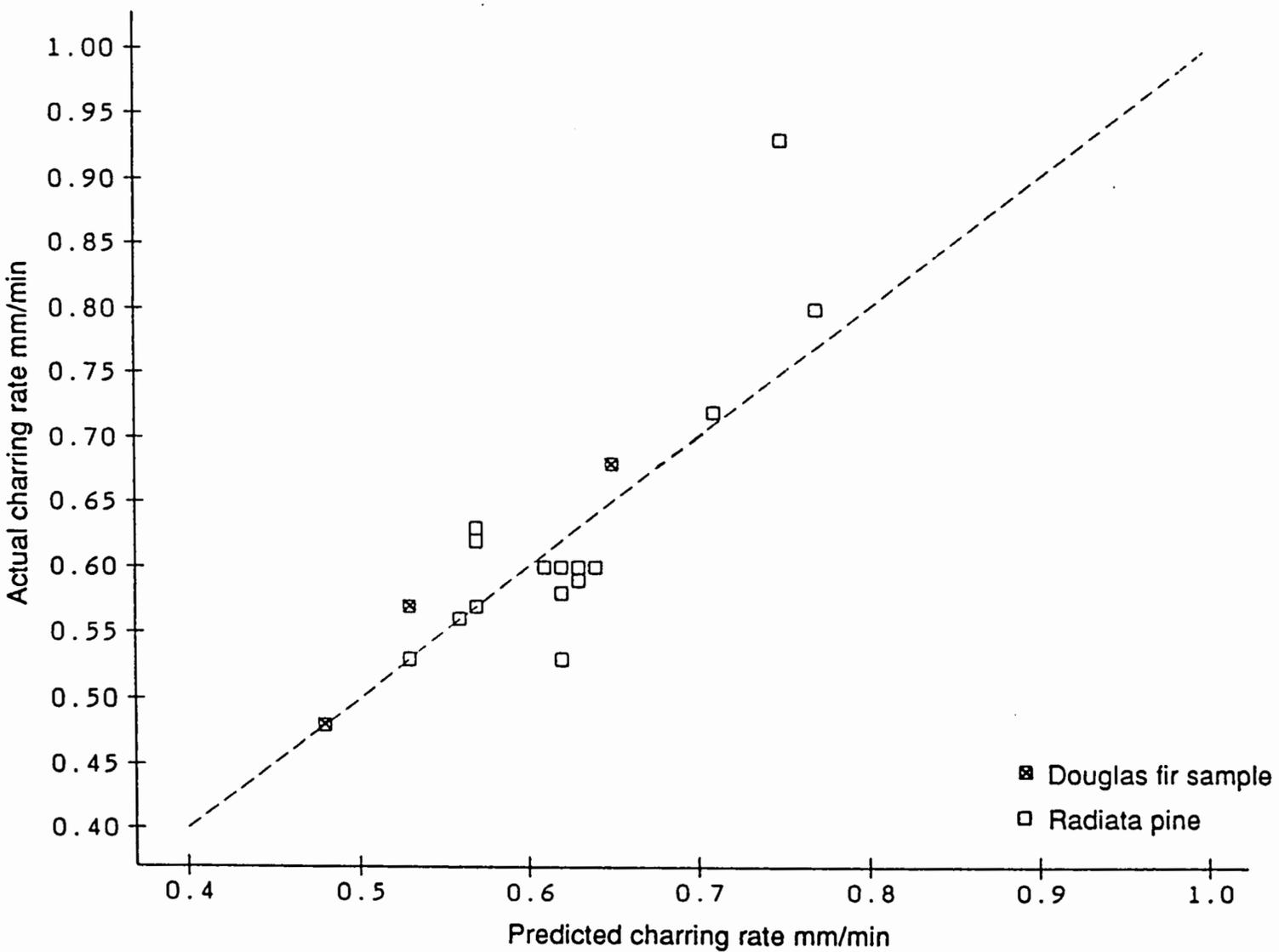
Figure 6.2 Scatter diagram of char rates for 60 minutes exposure
