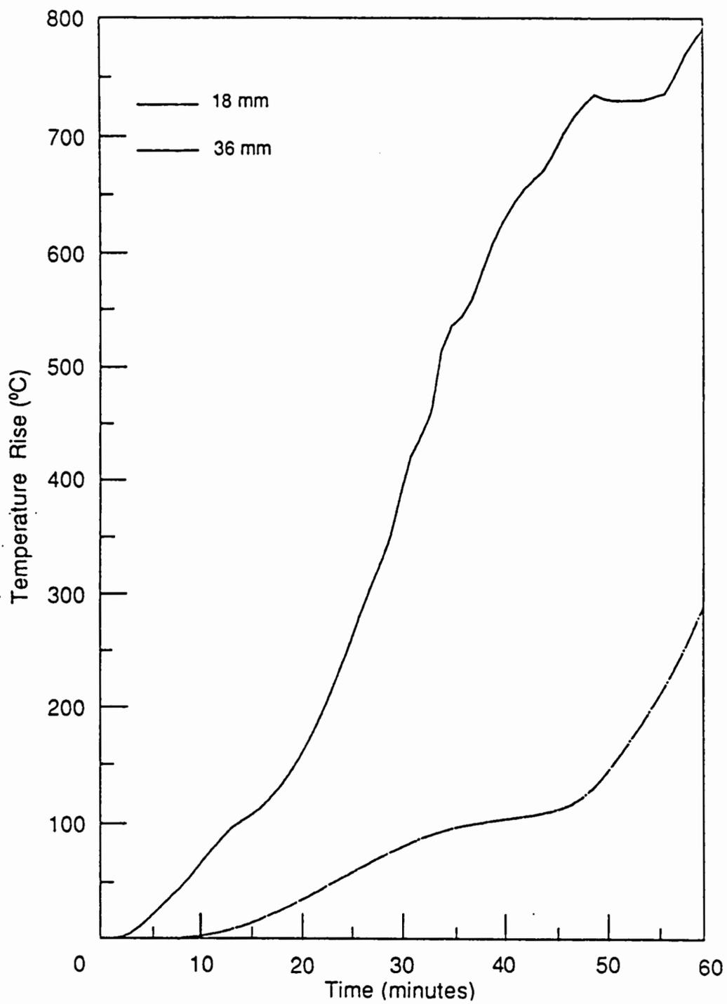
Figure 8 Temperature response of internal thermocouples 18 and 36 mm (ambient temperature 11°C)
