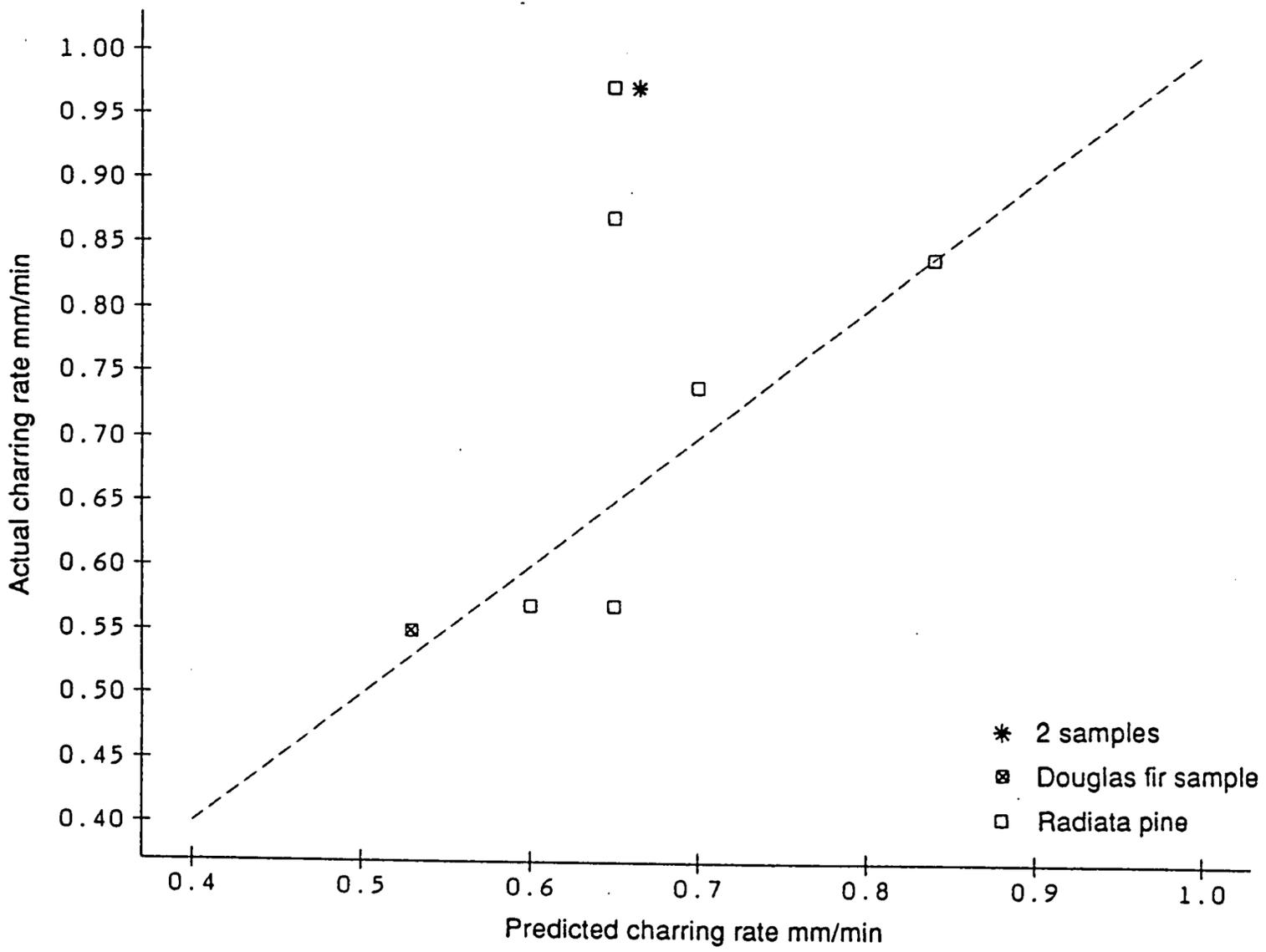
Figure 6.3 Scatter diagram of char rates for 29-60 minutes exposure
