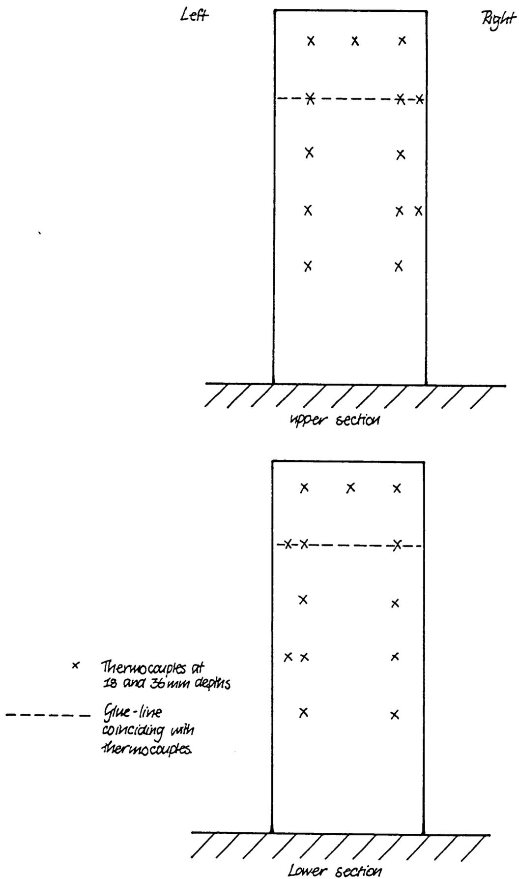
Figure 5 Location of thermocouples in glulam sections.
