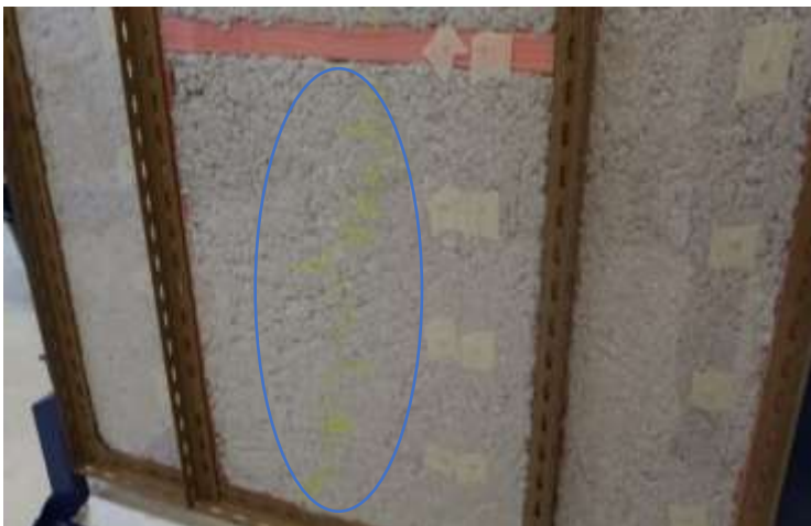
Figure 5. Example of water transfer to inside of loose-fill insulation. Water contains fluorescent yellow dye.
