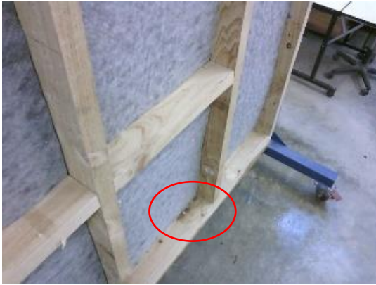
(a) Small amount of water was transferred to bottom plate with knot in it
