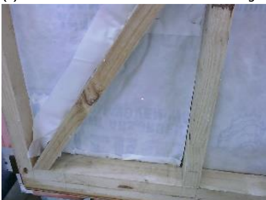
(d) Small amount of water was transferred onto corner of diagonal bracing and bottom plate
