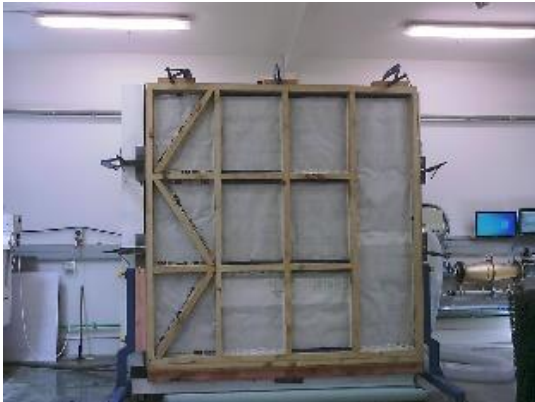
(i) Underlay taped to framing
