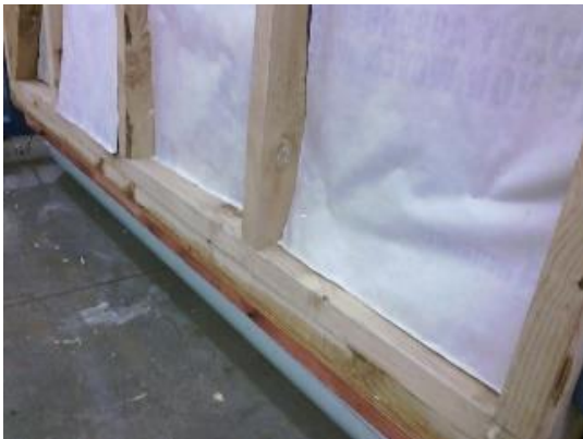
(f) Water was transferred to bottom plate
