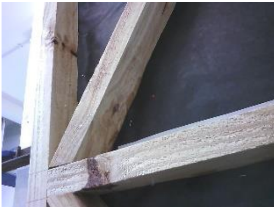
(f) Water was transferred onto diagonal bracing
