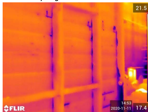
(d) Water was transferred onto framing and back of cladding
