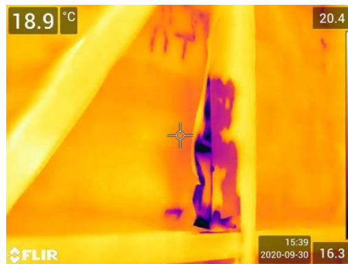
(c) Water was directed onto framing behind folded underlay edges
