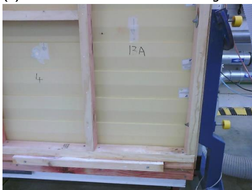
(b) No water was found at bottom plate of tall cavity
