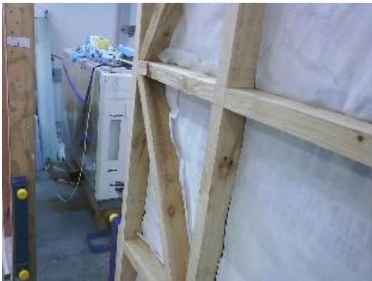
(b) Water was not transferred onto framing
