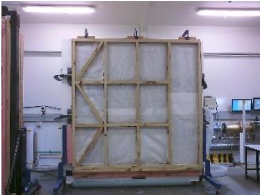
(a) Strip of synthetic underlay tucked between framing and back of cladding
