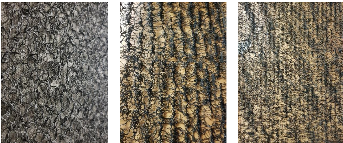
(a) 8 mm, integrated underlay (b) 7 mm, separate underlay (c) 7 mm, separate underlay
