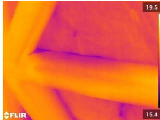
(b) Close-up view – water was transferred to bottom plate with knot in it
