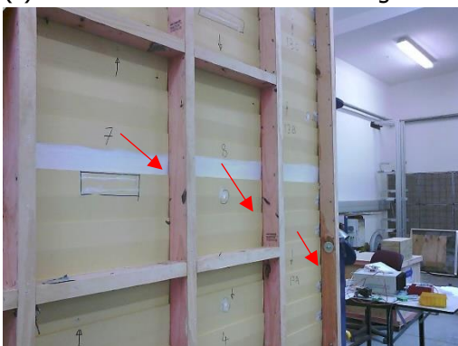
(d) Water was transferred onto framing and back of cladding
