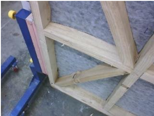
(d) Water was transferred to bottom corner of diagonal bracing and bottom plate
