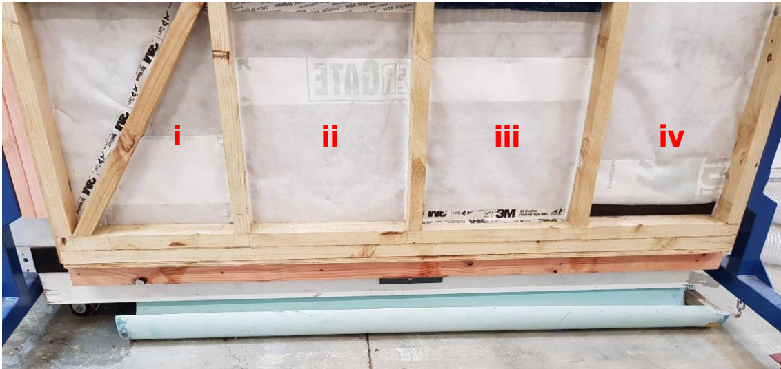
Figure A1. Four types of configurations were tested: i) the underlay was cut to fit the cavity; ii) the underlay was cut approximately 5 mm longer and tucked between the framing and the back of the cladding; iii) the underlay was taped to the framing; iv) strip of kraft paper was tucked between the framing and underlay. This image was taken before the test.
