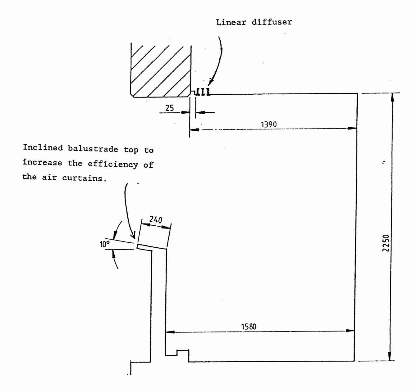
Figure 7Typical section through the balcony showing location of linear diffuserin relation to balustrade
