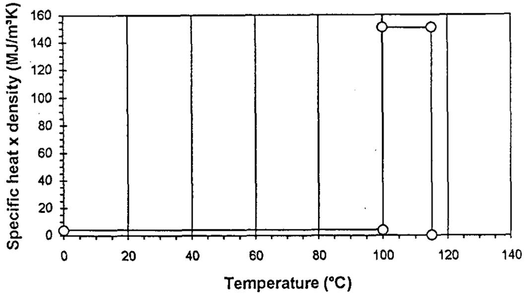
Figure 1 : Heat Capacity of Water
