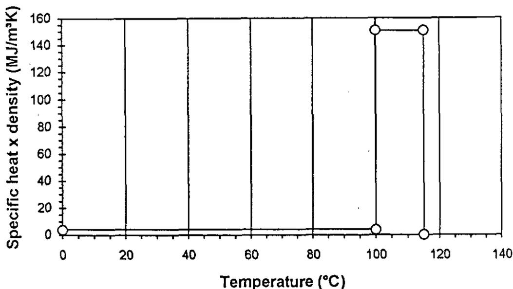
Figure 1 : Heat Capacity of Water
