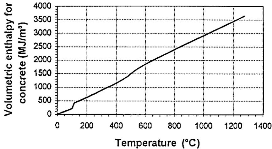
Figure 5 : Volumetric Enthalpy for Alluvial Quartz Concrete (Moisture Content 3.3%)
