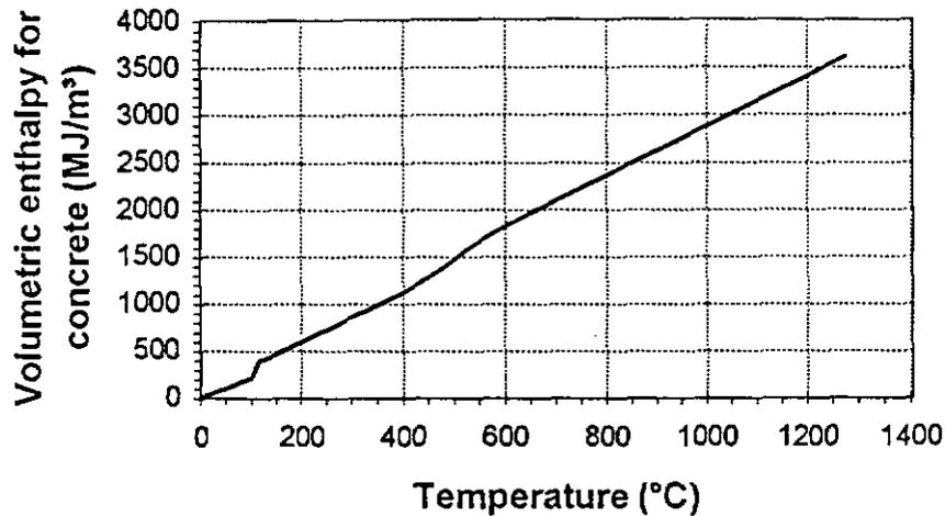
Figure 2 : Volumetric Enthalpy for Alluvial Quartz Concrete (Moisture Content 2.8%)
