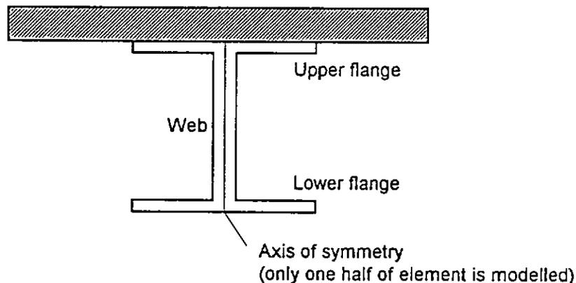
Figure 8 : Sketch of Steel Section and Floor Slab (not to scale)
