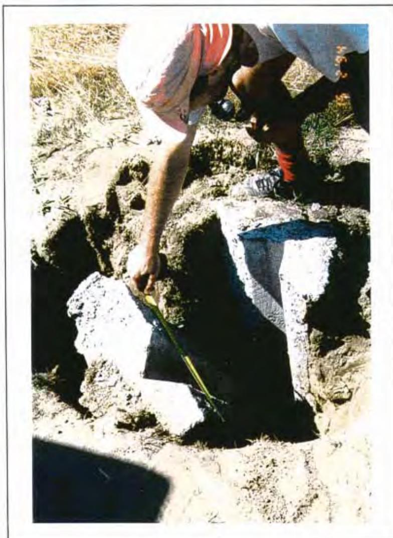
Figure 24. Failure of Footing at Pile M1 (photograph taken after the soil was dug away)
