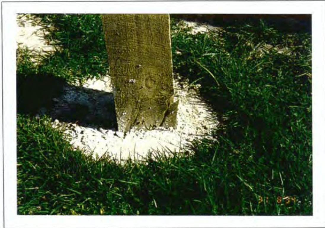
**Figure 23. Failure of Pile W13 in Flexure**
