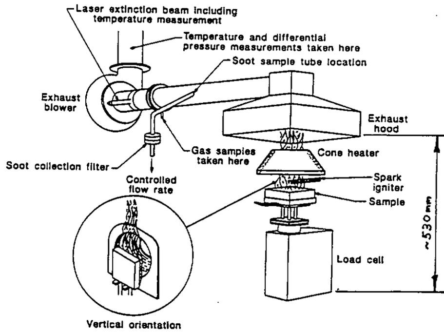
Figure 2 General Arrangement of the Furniture Calorimeter (NORDTEST, 1987)
