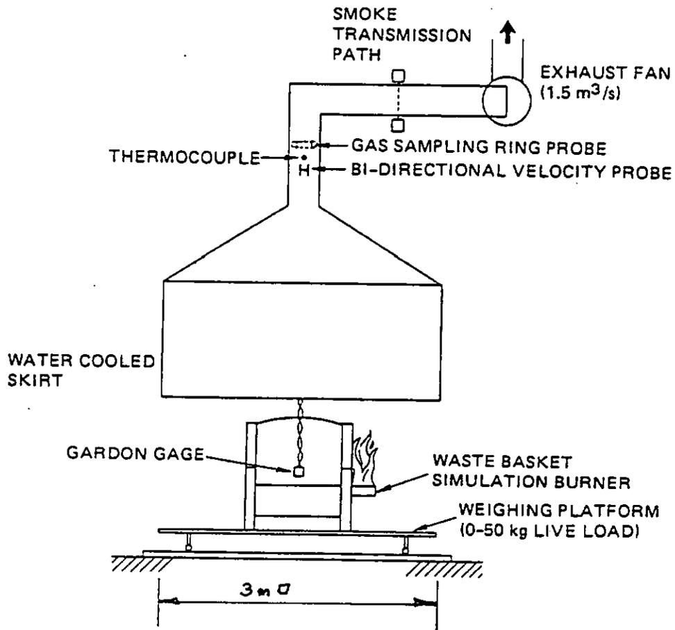
Figure 3 General Arrangement of the Cone Calorimeter
