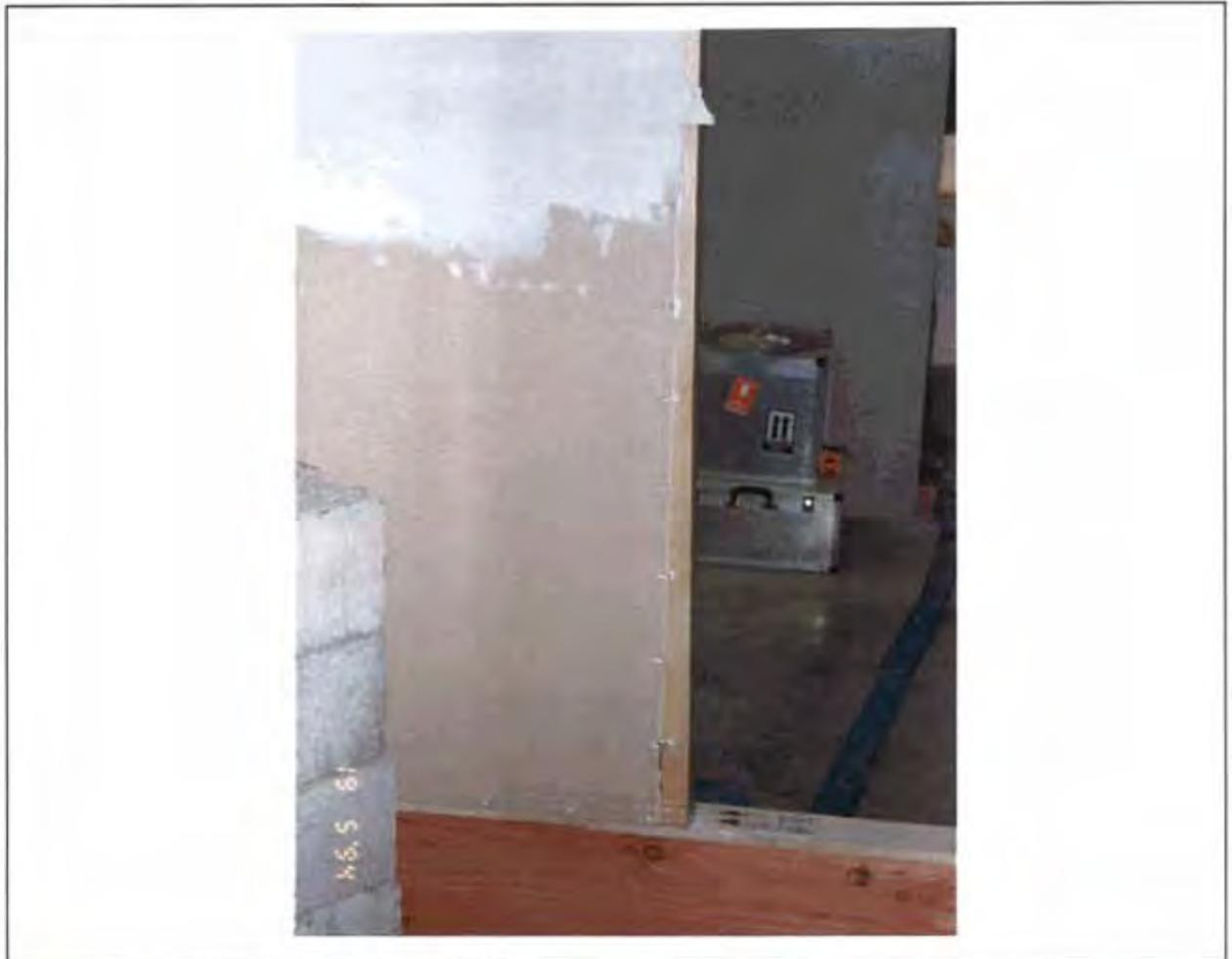
**Figure B7 Deformed shape of framing at +30 mm top plate lateral displacement.**
