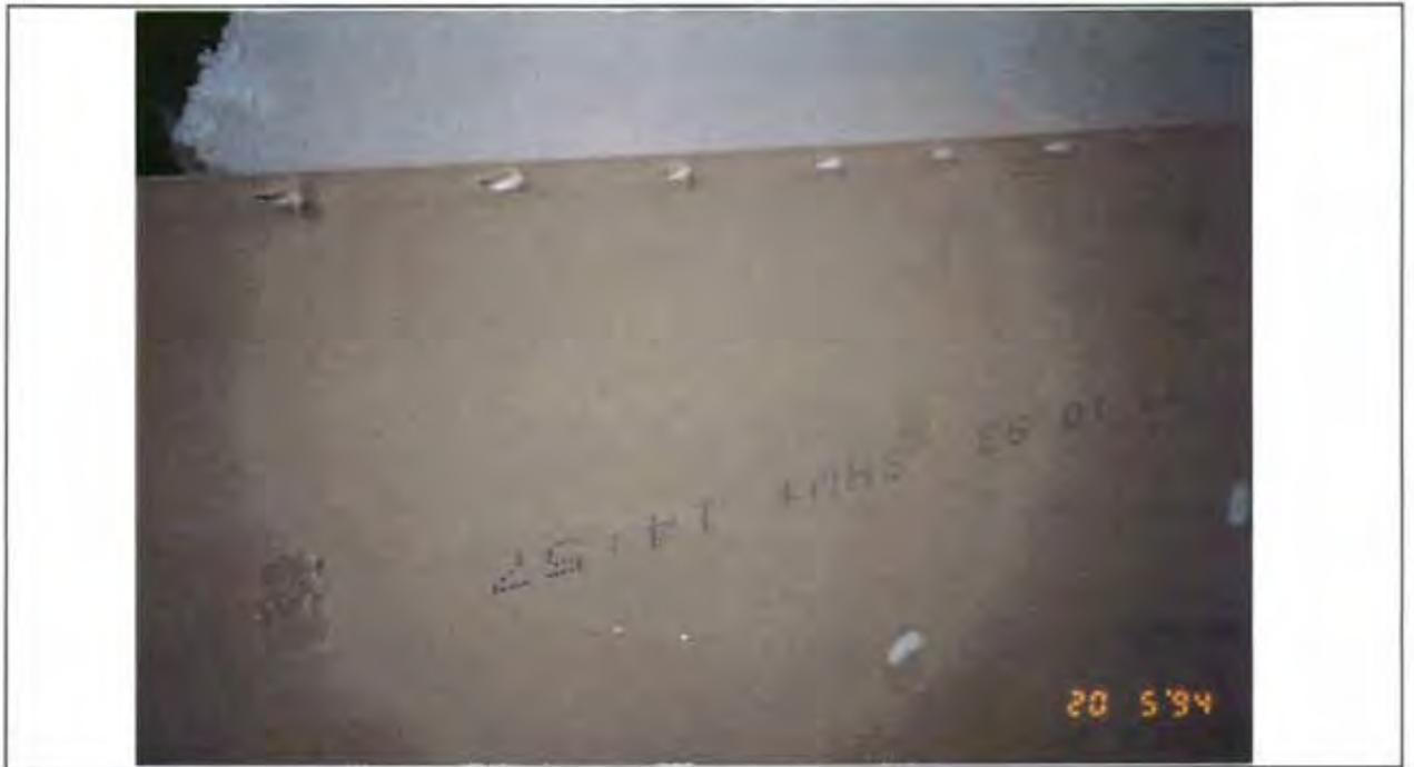
**Figure B9 Framing face of plasterboard after test.**
