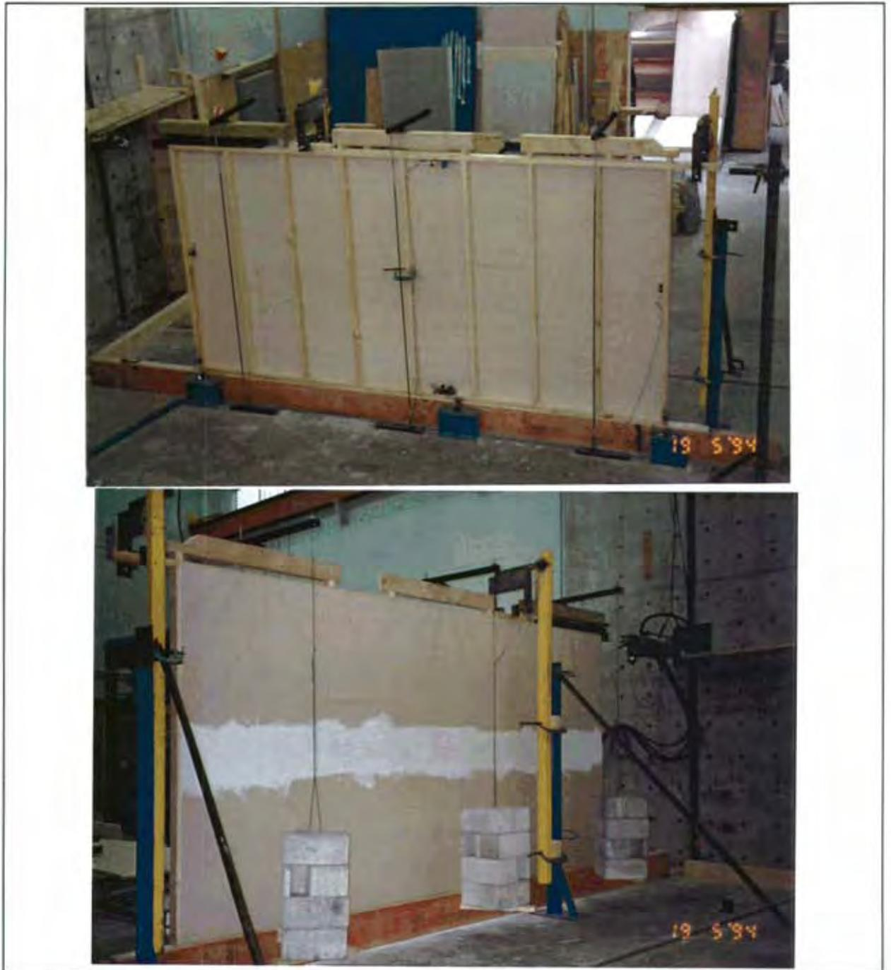
**Figure B4 Test arrangement for long wall specimens: a) Viewed from the framing face and b) Viewed from the plasterboard face.**
