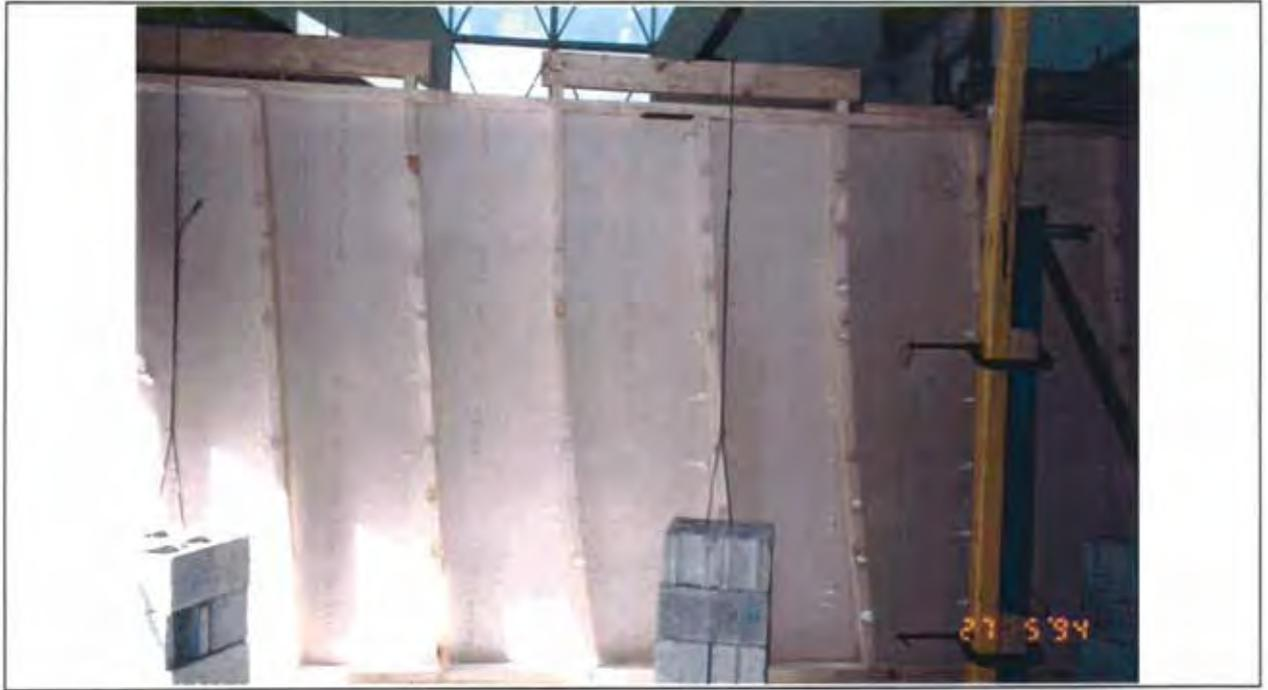
**Figure B13 Specimen LW2 at the end of the test (+290 mm displacement).**
