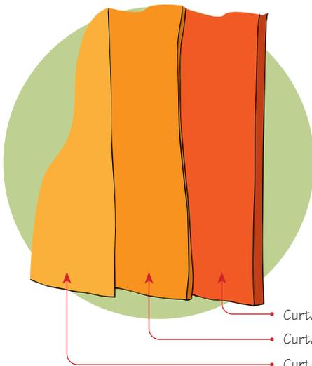
When we added thicker linings to the long curtain on a tight track, the camera showed the curtain was warmer than when it was lined with a thin sheet lining. This means that thicker linings help stop the curtain surface cooling down so it's not as uncomfortable to sit near. A thick lining can also hold more still air behind the curtain and slow down how much heat is lost through the curtain.
