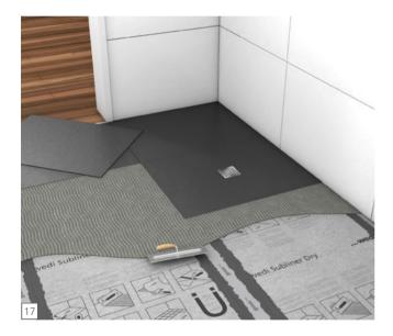
Before laying the tiles on floors, the adhesive must be fully cured underneath the sheet. Otherwise, unevenness can develop when the floor is being walked on.
