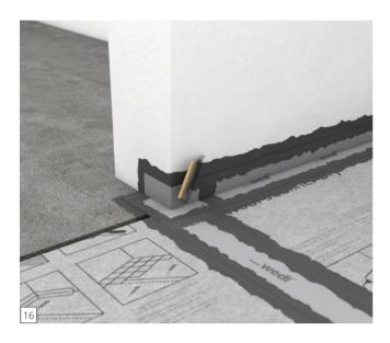
When sealing behind door frames, the correct wedi corner must be sealed in the corner area on the surface and with the adjacent sealing tapes, sealing membrane and wedi 620 sealant. There must be a minimum of 50 mm overlap.
